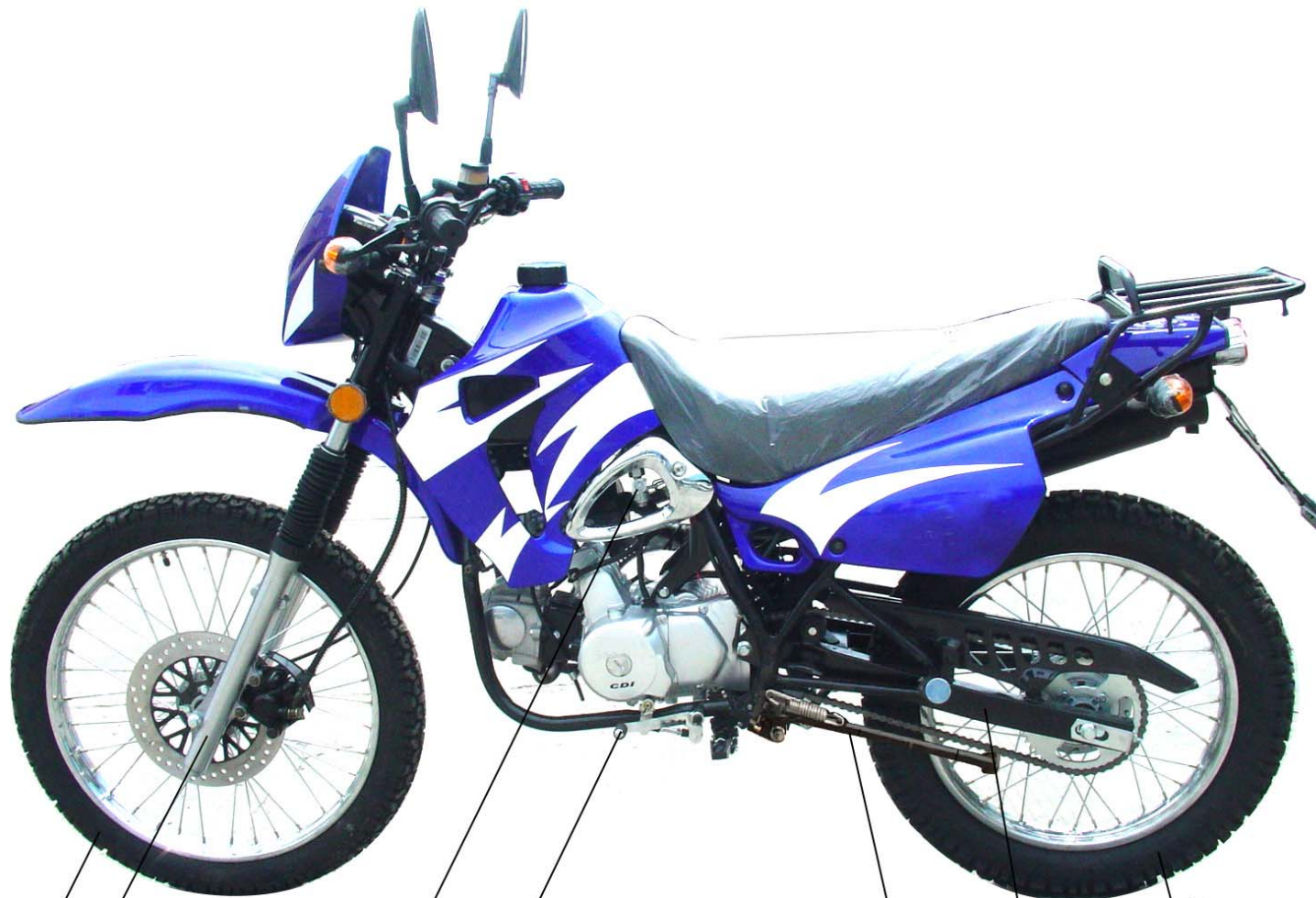
1. front wheel 2. front shock absorber 3. fuel tank 4. gear shifting 5. side stand 6. rear fork 7. rear wheel
