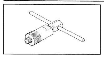
2. Flywheel Magneto Puller P/N. YM-01189
