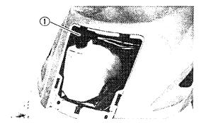
NOTE: \_\_\_\_\_\_ Install the oil tank filler cap ① and push it fully into the filler.
