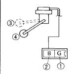
Check the fuel sender for specificated resistance.
