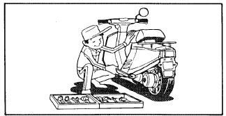
3. When disassembling the scooter, keep mated parts together. This includes gears, cylinders, pistons and other mated parts that have been "mated" through normal wear. Mated parts must be reused as an assembly or replaced.
