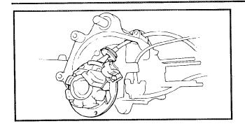
3. Pass the C.D.I. magneto lead through the crankcase hole.
