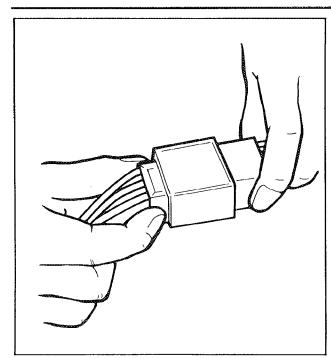
1. Disconnect the main switch coupler from the wireharness.
