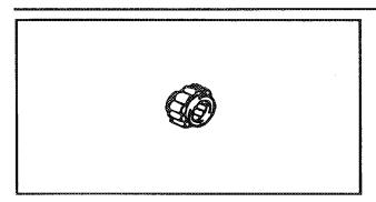
4. Inspect:Bearing (piston pin)Pitting/Damage → Replace.
