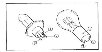
3. Check the bulb socket by installing a proven bulb to it. As in the checking of bulbs, connect the pocket tester leads to the respective leads of the socket and check for continuity in the same manner as mentioned above.
