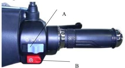
A. Headlamp Switch: When this Button is pushed to the leftmost position, all lights are switched off; When the Button is pushed to the middle, the Position Lights both at front and rear will be turned on; When this Button is pushed to the rightmost position, headlamp starts to work.
