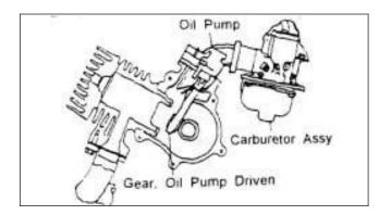
B. Oil-Pump: Double outlets type , The Injection Volume Increased by The Revolutions of Crankshaft and The Opening of Throttle.
