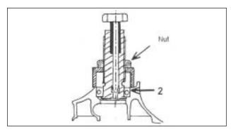
H. Put the crank case on the spacer shown. Push the outer ring of the bush with another spacer.And press the bush out with a vice.
