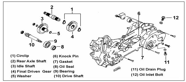
A. Apply a little gear oil (GA50400004) on the right hand bearing of rear axle, and then evenly press into the reducing gear chamber. with fixture.
