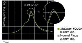
Vehicle: 1600cc 4 cylinder Conditions: 1200rpm - 60KPa 0.4MPa/DIV average ripple mark of 256cycle Note Iridium Tough increases combustion pressure and output
