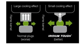
The fine electrode has a smaller cooling effect on the flame kernel
