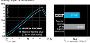
Vehicle: 250cc (2 cycle water cooled, 2 cylinders Conditions: 50km/h, then accelerating for 27 seconds at full throttle (locked in 4<sup>th</sup>)
