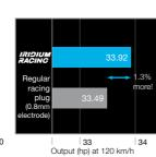
Vehicle: 250cc (2 cycle water cooled, Conditions: WOT 60 to 120km/h Data: In-company Comparisor
