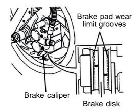
check the brake from behind the brake caliper.
