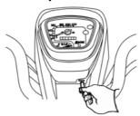
Engine oil replacement indicator is used to indicate the time tables of engine oil replacement, the color is expressed as green as usual. When the vehicle traveling about 1,000 kilometers, the indicator light turns red. It means that it need to supply or replace engine oil.
