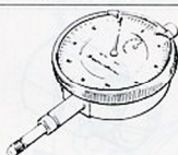
Dial gauge 09900-20606 (0 ~ 10 mm, \frac{1}{100} mm)
