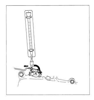
Holding engine speed at the 2 000 r/min by turning the throttle stop screw, move the lever up to the fully open position and let the pump draw for 6 minutes. For this operation, the reading taken on the measuring cylinder should be from 1.02 to 1.26 ml.
