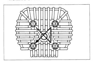
Cylinder head nut 0.8 - 1.2 kg·m (6.0 - 8.5 lb-ft)tightening torque
