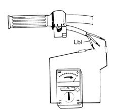
Check the conductivity between the lead terminals on the left handle switch box when the turn signal indicator knob is operated.
