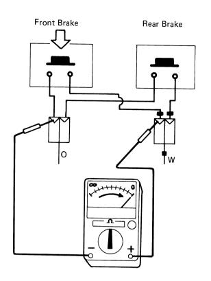
• Place the pocket tester between orange lead wire and white lead wire with the red tube and squeeze the brake lever. If continuity is found, it is in good condition. If not, replace it.
