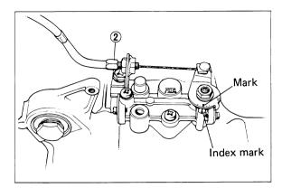
If the marks are not aligned, adjust by means of the cable adjuster ② to align them.
