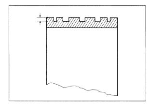
Inspecting clutch shoe groove.
