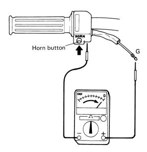
Connect the lead wire in the headlight housing and the ground wire to the pocket tester, set knob range to R and press the horn button. If continuity is found, it is in good condition.
