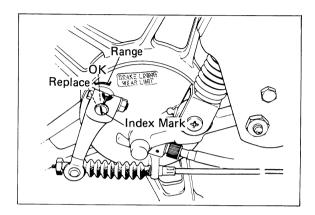
Remove inspection cap on the rear hub panel and check the brake shoes. If they are worn as much as the limit shown in the figure below, replace them.
