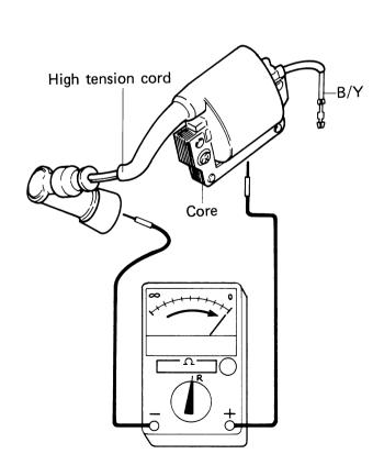
• Using the pocket tester check the ignition coil.
