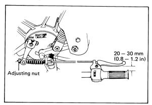
• As the rear brake wire is linked to the kick starter lifter lever, first adjust with the adjusting nut so that the lifter lever play is 1 mm (0.04 in).
