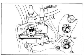
Check whether the mark on the oil pump control lever is aligned with the index mark when the throttle valve is positioned as above.
