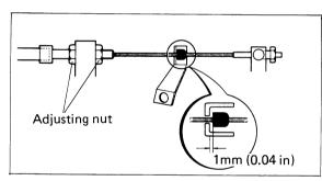
• Adjust by turning the brake cable adjusting nut so that the clearance between lever and grip is 20 - 30 mm (0.8 - 1.2in).
