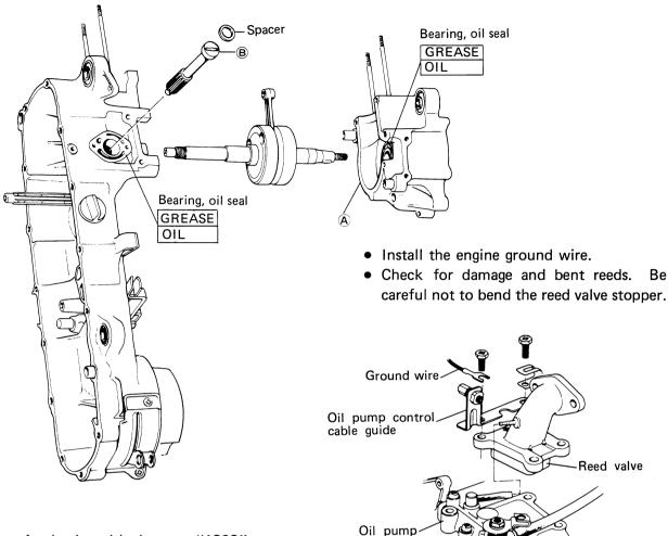
• Apply thread lock super "1303" to outer surface of right oil seal.
