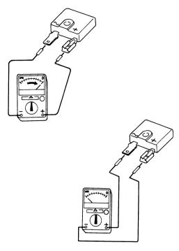
• If continuity is found in  $\Omega$  range when connecting as shown in the figure and not found when (+) (-) probes are reversed, it is in good condition. If continuity is found in both cases or no continuity in either case, replace it.
