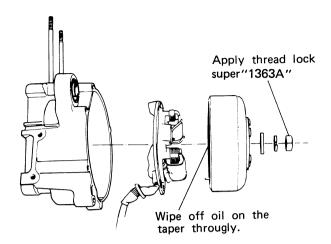
Fix the stator to align the scribed line with the center of the screw hole so that correct ignition timing is assured.
