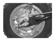
(3)Adjust the sag of transmission chain by turning the adjusting bolt to the right or left.At the same time, the centers of the front and rear sprockets must be held in alignment. For your convenience of adjustment, reference marks are made on swing arms and all chain adjusters. They can be aligned with each other and referenced from one end to another Refit the locking nut(1) and lock the adjusting nut(2) after the sag of transmission chain is adjusted between 15-25 mm.
