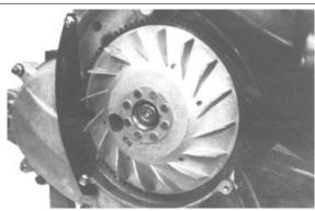
Using the appropriate tool, unscrew the lock-nut of the flywheel.
