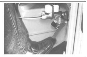
Lower the pedal, keeping it pressed, undo the bleed screw on a rear wheel, let the air out, after this bleed point has been connected through a small rubber pipe to a tray full of brake fluid. Screw the bleed screw.
