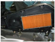
If there is too much accumulation of dust inside the air cleaner, it will reduce the output of engine performance and cause abnormal consumption of fuel.
