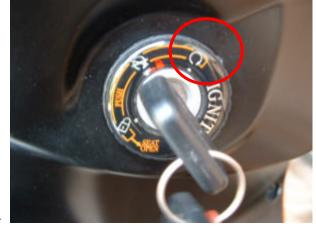
Please do not push the button over 5 seconds per each time. Try kick starter to start the engine if the start button is not working properly.
