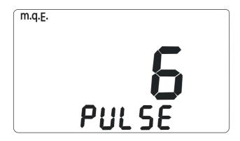
Pressing the control button for more than 3s will allow you to set the number of pulses per wheel revolutions.
