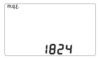
Press the control button (for more than 3s) until the screen displays only the wheel circumference.
