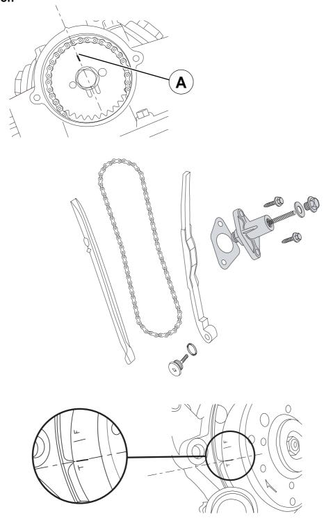
Single overhead camshaft driven by a noiseless chain from the crankshaft. Automatic chain tensioner.
