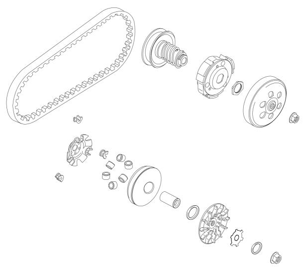
Fixed flange of the pulley equipped with cooling fins to cool the belt.
