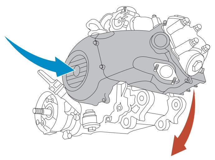
By a circulation of forced air by means of a turbine on the flywheel magneto.
