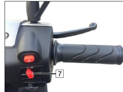
5. Right switch(7) at " ⤵ "position.
