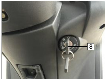
6. The ignition key(8) at "↷" position.
