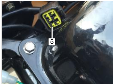
3. Fault diagnosis tester connector (5).
