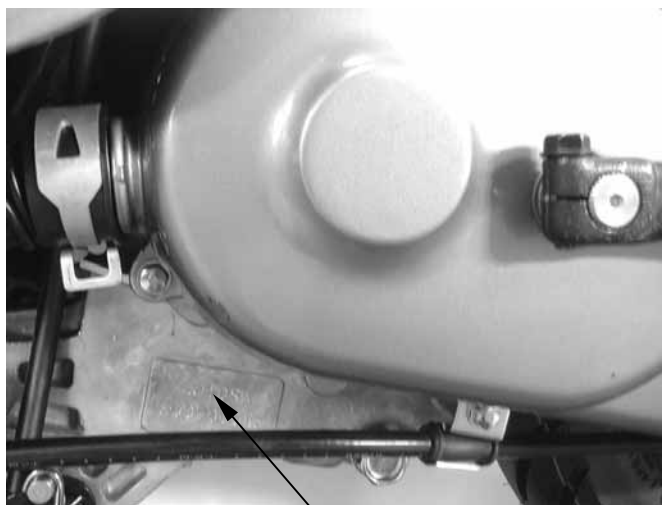
Location of Engine Serial Number
