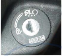
Shut off the turn signals and turn the ignition key to OFF position after parking well the motorcycle.
