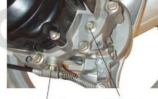
Draining bolt Filling hole of gear oil of gear oil
