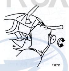
Rotate accelerate, it is better to rotate slowly Return, It is better to return quickly
