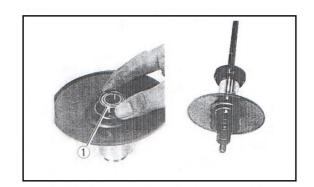
• install the spacer ② and circlip③.
