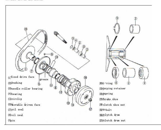
• install the bearing② in the fixed driven face① with the special tool.
