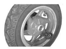
When installing this speedometer gear box, align the two driving pawls with the two recesses of the wheel hub.
