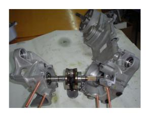
• disassemble crankcase with special tools
