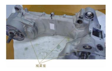
Install shock absorber bushing
