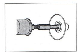
**CAUTION:** Replace the removed bearing with a new one.
