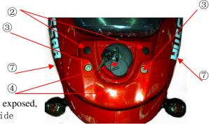
3. unlock oil pump cap and remove it, two tapping screw are exposed, remove them; remove tapping screw@; then remove side cover:
