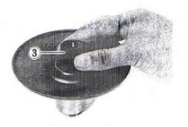
• Install the bearing ① with special tool
