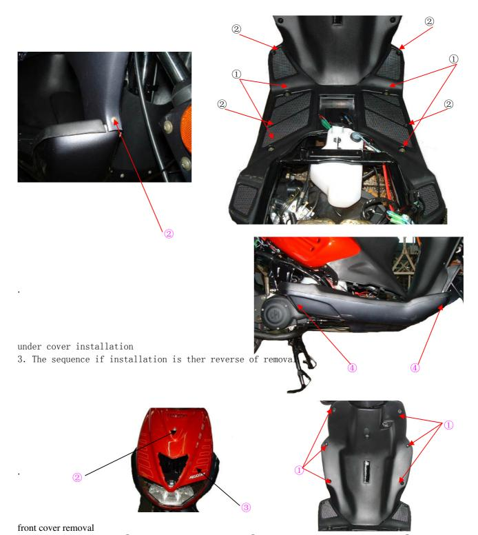
1. Unscrew tapping screw①, and remove front cover③ by removing front cover screw②
