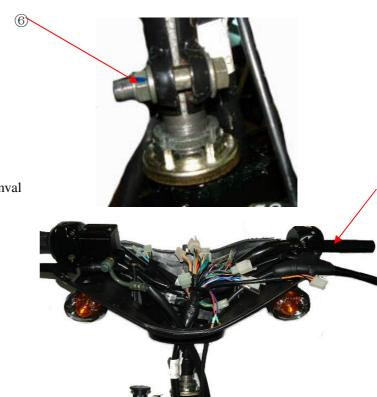
Handle cover unstallation 7. The sequence of removal is the reverse of reomval
