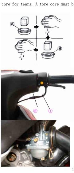
Connect an electric tachometer to the connecting protiion of the magneto lead wire as shown I nthe illustration. Use the selector key "C' position.
