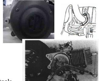
• Remove magneto nut with special tools.
