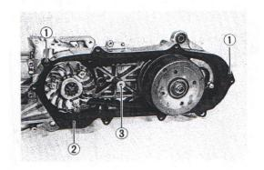
apply QIANJIANG bond no. 1215 to the clutch cover as shown in the illustration. QIANJIANG bond no. 1215
