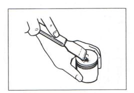
be taken in the intake-to-exhaust port direction and at 20mm from the cylinder top surface.
