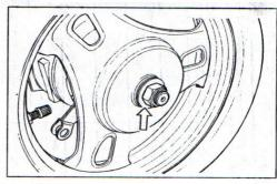
• remove brake shoe 5 and rear axle 6.
