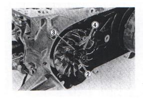
• continue turning the fixed drive face by hand until the belt is seated in and both the drive and driven faces will move together smoothly with slip.
