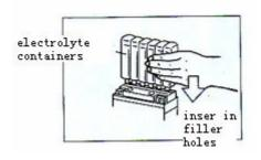
• Make sure air bubbles are coming up each electrolyte container, and leave in the position for about more than 20 minutes.
