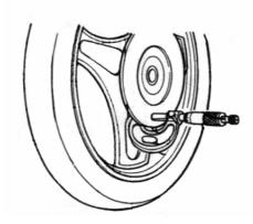
With the disc mounted on the wheel, check the dids for face runout with a dial gauge as shown.
