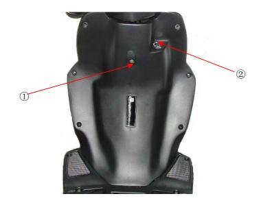
3. remove legshield and pedal by unscrewing the four bolts(3)
