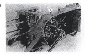
• fill grease in the groove provided inside sliding surface of the kick driven gear and install ② on the end of the crankshaft. Wipe pff excess grease.
