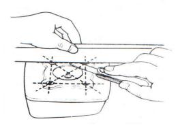
If the largest reading at any portion of the staightedge excees the limit, rework the surface by rubbing it against emery paper laid flat on the surface plate in a lapping manner. The surface must
