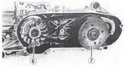
• fill the final gear box with engine oil up to the level hole.
