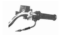
Remove the brake lever and brake switch.
