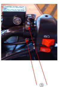
3. Disconnect throttle cable  $\ensuremath{ \Im}$  and oil pump cable  $\ensuremath{ \Phi}$
