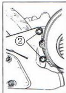
• lubricate brake cam shaft with QIJIANG SPECIAL grease.
