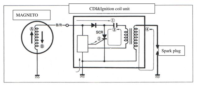
The ignition system consists of a flywheel magneto, a CDI&Ignition coil unit and a spark plug.
