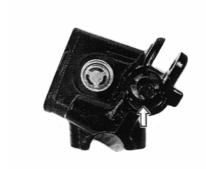
Remove the piston/primary cup with return spring. Remove the reservoir cap and diaphragn. Drain brake fluid.
