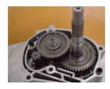
• install gearcase cover into crankcase and lock bolt.
