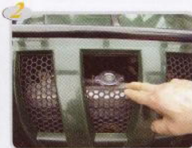
Open the radiator cap and add the water
