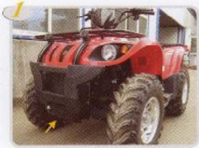
1. Winch located here
