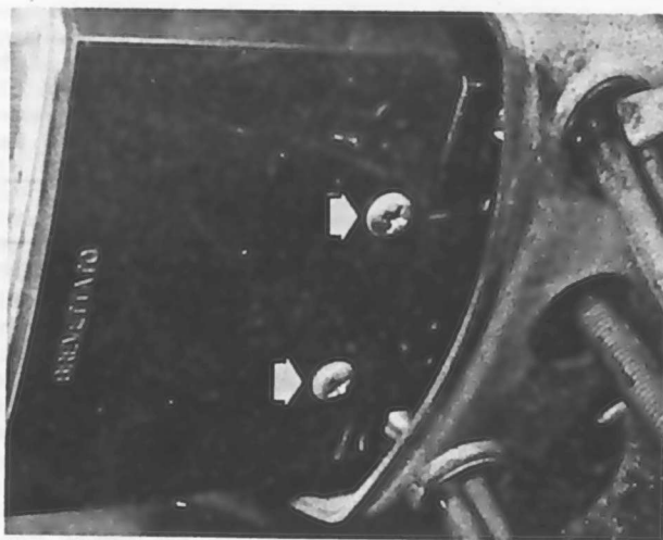
3.1b Earlier type has securing screws only (arrowed)
