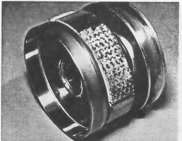
29.2c Examine condition of linings
