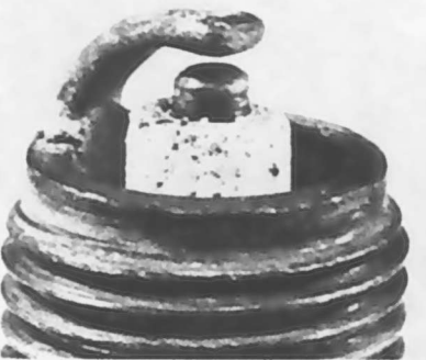
A blistered white insulator or melted electrode indicates over-advanced ignition timing or a malfunctioning cooling system. If correction does not prove effective, try a colder grade plug
