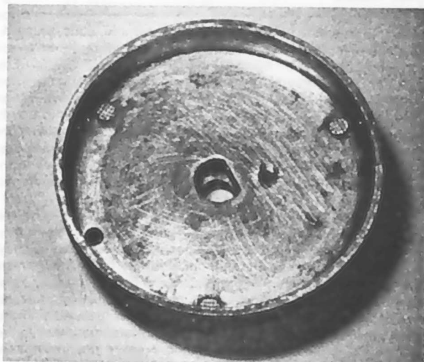
23.4b Backplate forms drum for starting shoes
