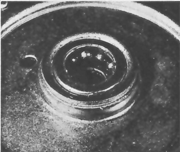
5.3 Balls are retained by steel ring
