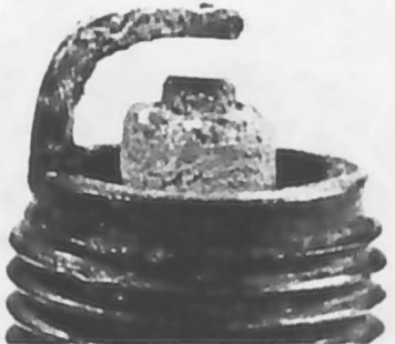
A worn spark plug not only wastes fuel but also overloads the whole ignition system because the increased gap requires higher voltage to initiate the spark. This condition can also affect air pollution
