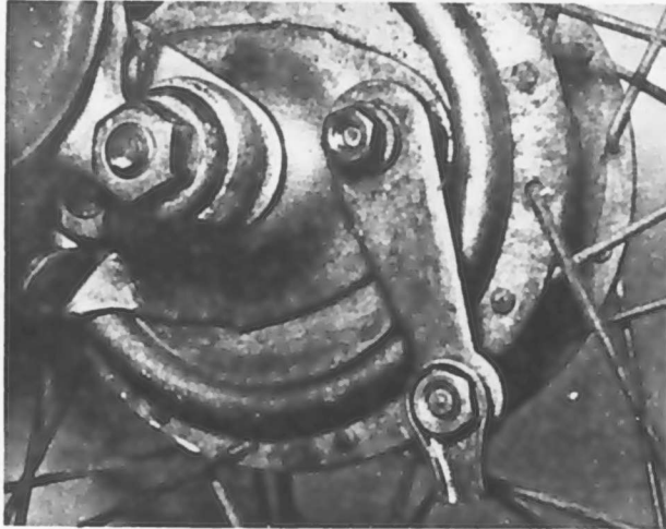
3.2 Release front brake cable and wheel nuts
