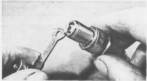
Altering the plug gap. Note use of correct tool
