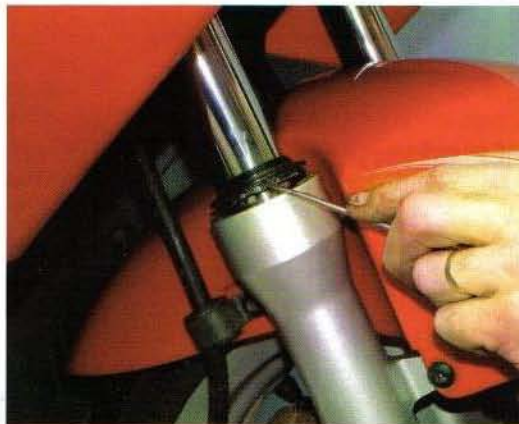
When prising up dust covers to check oil seals, take care not to damage the soft plastic or rubber
