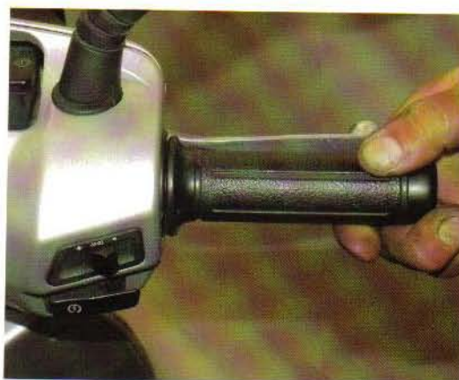
Checking throttle freeplay at the handlebar end. Throttle action should be smooth and should willingly snap shut when released
