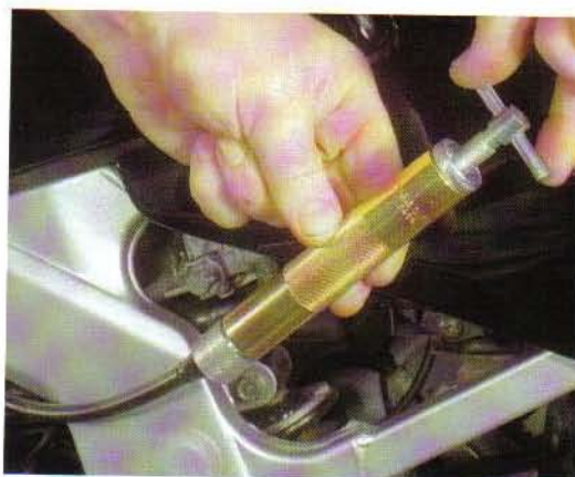
Pressure lubricator forces light oil in between the cable inner and outer
