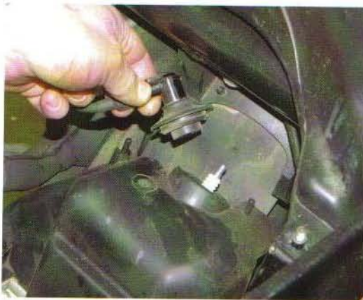
The spark plug(s) may be well hidden away for protection from the elements, but make plugs a regular part of your maintenance schedule
