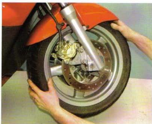
Checking for front wheel bearing wear with the wheel off of the ground
