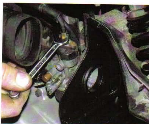
Taking up the slack in a throttle cable at the carburettor end. Take care not to take up so much that the idle rises or the throttle can be operated when the bars are moved from side to side
