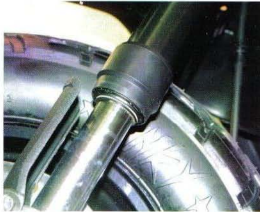
Even with a guard as fitted here to repel road dirt, it still gets on the stanchions and can lead to seal wear. Keep those shiny bits clean
