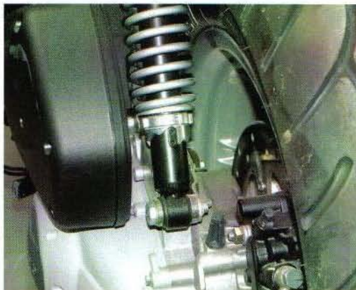
A plastic shroud on some shocks between spring and damper prevents dirt getting to the more sensitive moving parts
