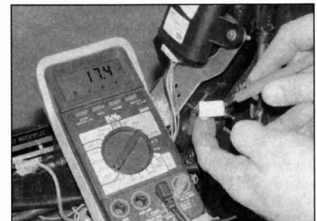
4.6c Measuring the resistance in the transponder aerial
