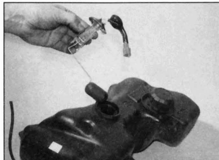
19.4d . . . and withdraw the sender
