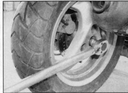
15.3 ... then loosen the hub nut
