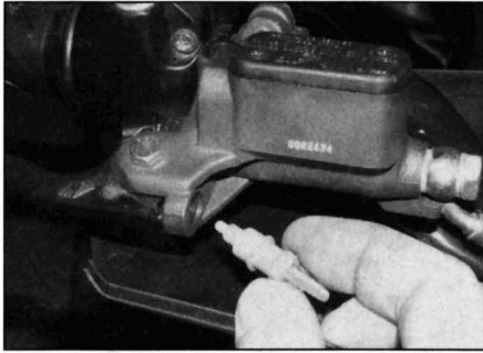
11.5 Switch screws into brake lever bracket
