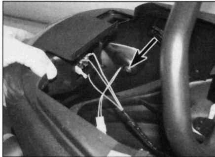
15.5 Retaining bolt for turn signal is inside rear cowling
