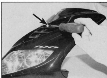
6.12a Grille is retained by central screw . . .
