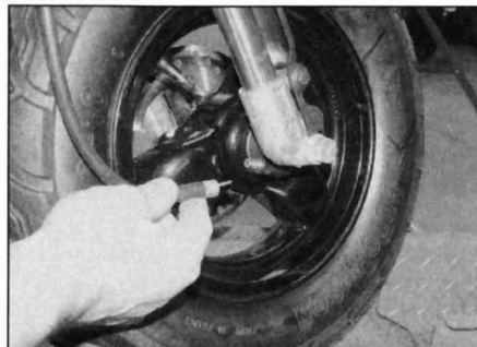
14.15 Disconnect the speedometer cable
