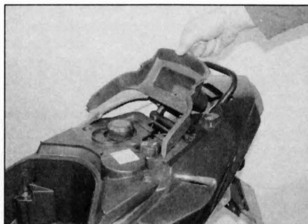
4.9 Remove the tool tray fitted to Speedflight models
