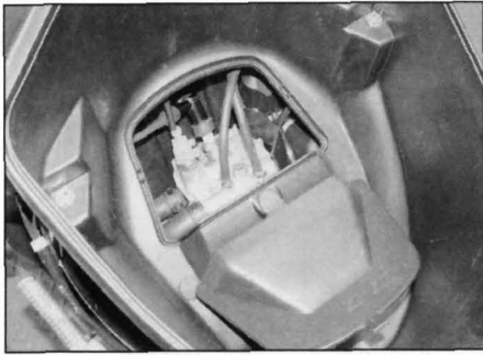
17.1a Open the engine access panel . . .
