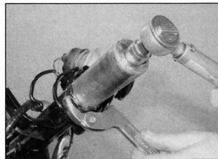
6.13 Hold the adjuster nut and tighten the locknut with the special tool
