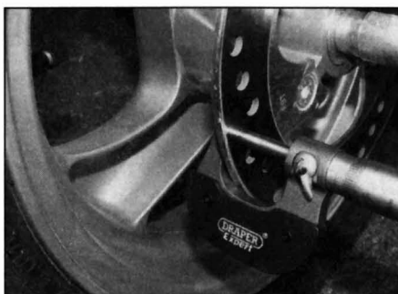
4.2 Measuring the thickness of a disc with a micrometer
