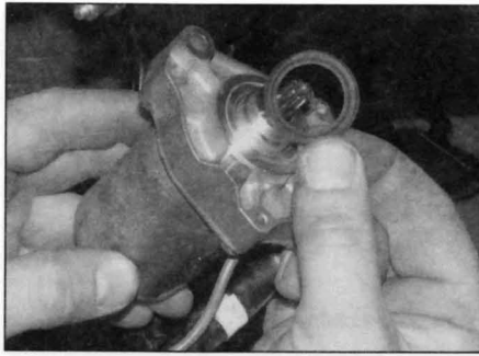
26.4 O-ring is fitted to starter motor body
