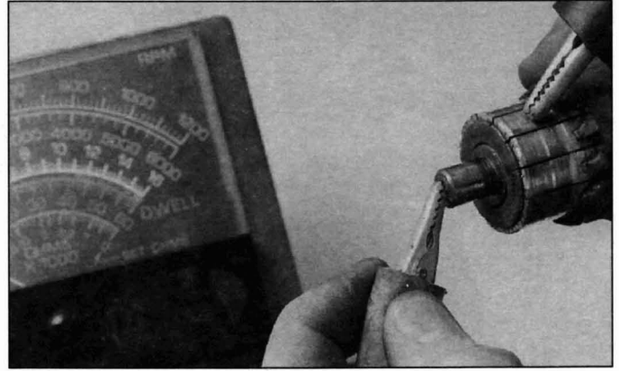
27.10 There should be no continuity between the commutator bars and the armature shaft
