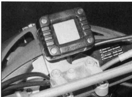
16.2b All-electronic instrument cluster as fitted to Speedfight 2 Furious and Metal-X Furious models
