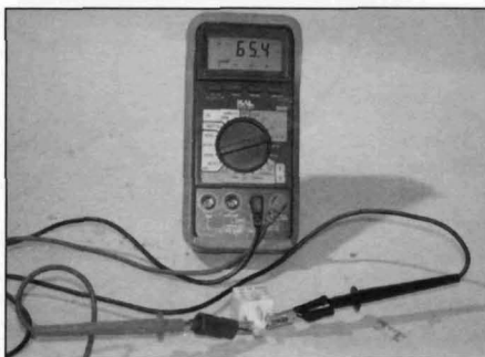
25.3 Measuring the starter relay primary resistance
