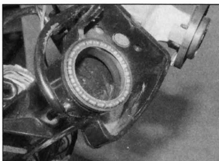
7.9 Install the top bearing
