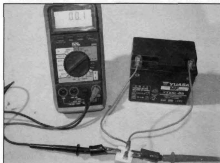
25.4 Measuring the starter relay secondary resistance
