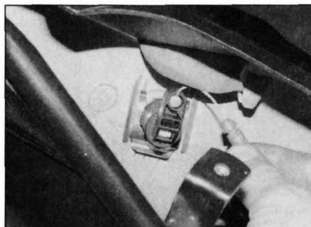
4.3d ... then from the back of the lock
