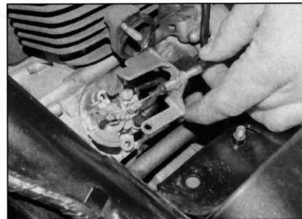
5.10 Remove the oil pump cable and bracket
