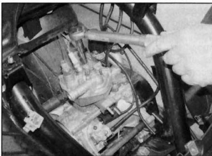
7.4 Undo the cylinder head bolts . . .
