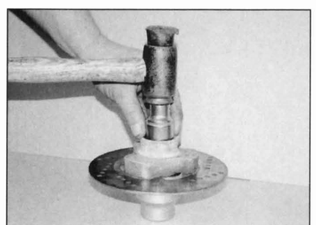
16.8 Installing a new bearing
