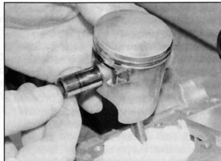
9.3b . . . then push out the piston pin
