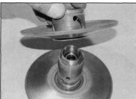
6.9b . . . and separate the pulley halves
