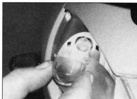
14.11a Unclip the bulb cover . . .
