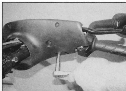
6.4a Undo the lower cover fixing bolts ...
