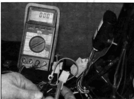
32.2 Checking for continuity in the regulator/rectifier earth (ground) circuit
