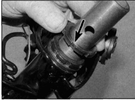
6.7 Remove the locknut (arrowed) and discard the lockwasher
