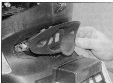
6.48b . . . and lift off the Boa lock panel
