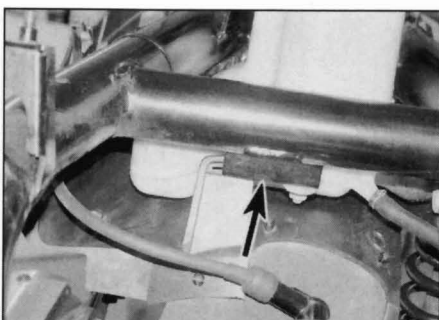
6.49b . . . and a lug on the frame
