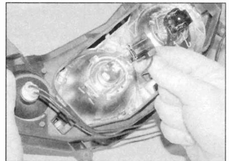
7.2a Remove the wiring connector ...
