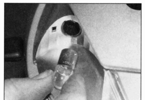
14.11b . . . and remove the bulb
