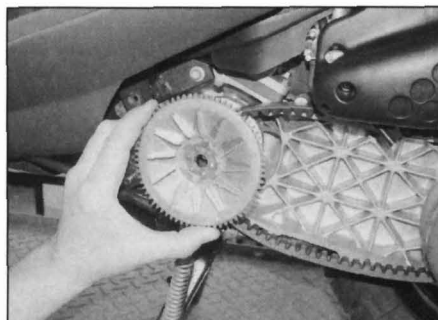
4.22a Install the outer pulley half . . .
