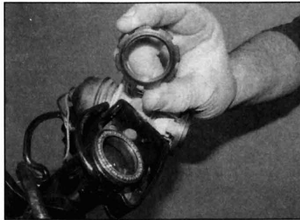
7.11b ... and install the adjuster nut
