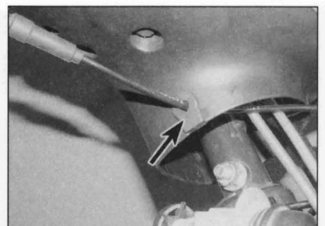
6.4b ... and detach the throttle cable
