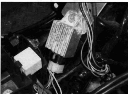
32.1 Location of the regulator/rectifier
