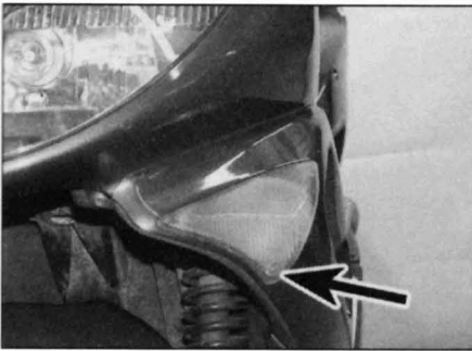
14.1a Retaining screw on front turn signal lens
