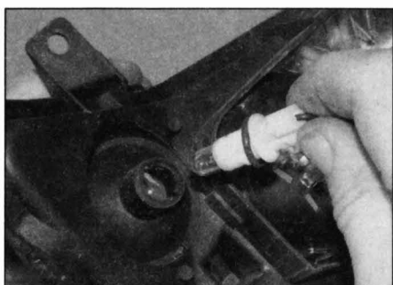
7.6a Pull the bulbholder out of its socket ...
