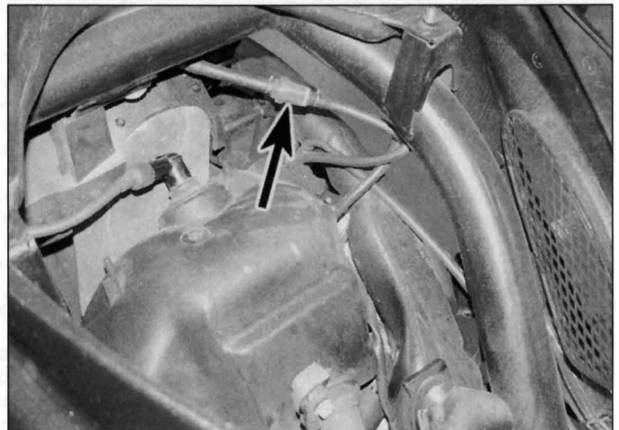
11.4 Inspect the oil filter (arrowed)
