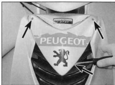
6.6a On Speedfight 2 models, undo the three screws (arrowed) . . .
