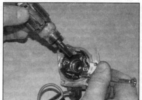
27.4 . . . then withdraw the armature from the cover
