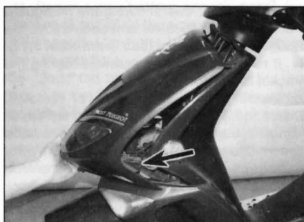
6.10a Pull the panel forward to disengage the tabs (arrowed) . . .
