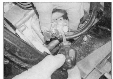
13.19b Bleeding a cable operated oil pump
