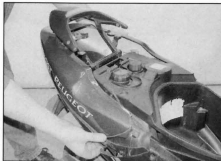
6.44 Ease the cowling off carefully
