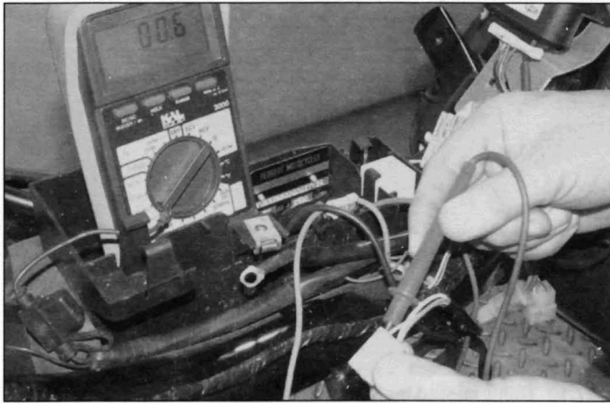
30.3 Checking the resistance in the alternator lighting coil
