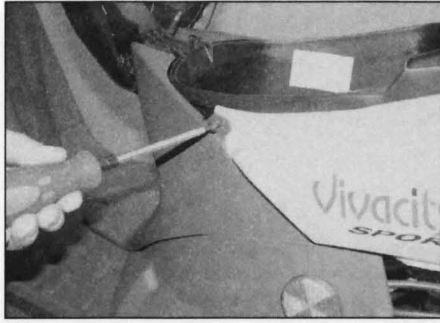
5.5 Battery panel screws also retain front of seat cowling
