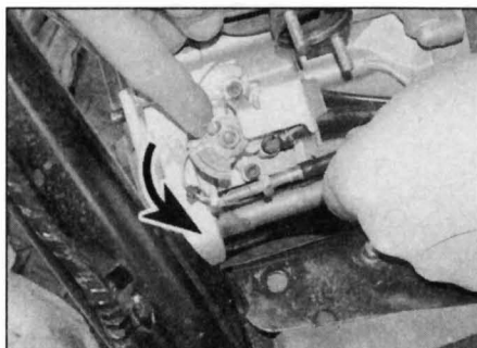
13.2 Rotate pulley to detach the oil pump cable
