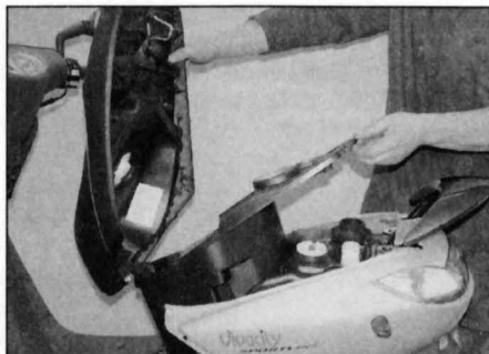
4.11b Lift the assembly off the machine
