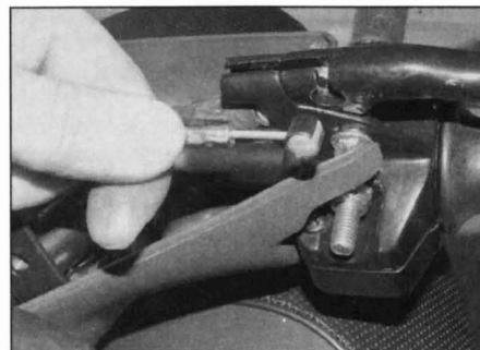
10.4b . . . and release the nipple from the lever
