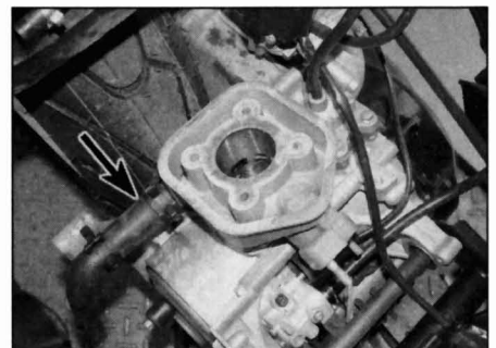
8.2 Detach the coolant hose (arrowed) from the cylinder
