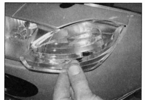
14.10b . . . then unclip the lens
