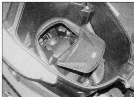
4.7 Engine access panel in the bottom of the storage compartment
