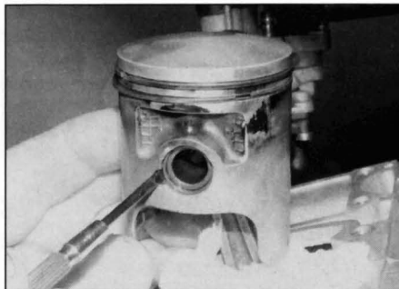
9.3a Remove the circlip . . .
