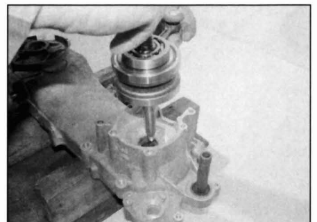
14.29a Fit the crankshaft into the left-hand crankcase half first
