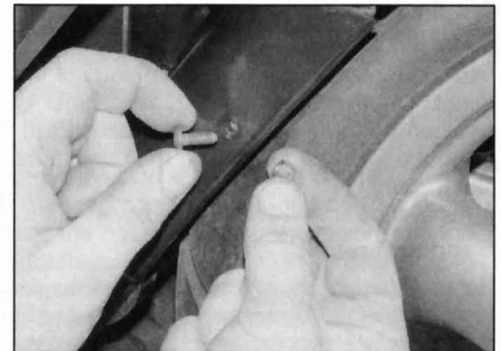
6.18 Mudguard is retained by two nuts and bolts on right-hand side . . .
