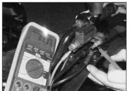
11.2b Testing the continuity of the brake light switch
