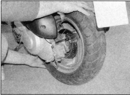
15.6b Slide the wheel off the axle . . .
