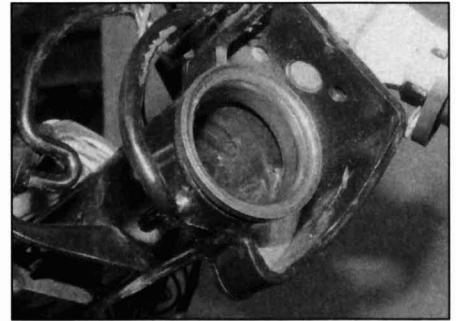
8.3a Inspect the races in the top ...
