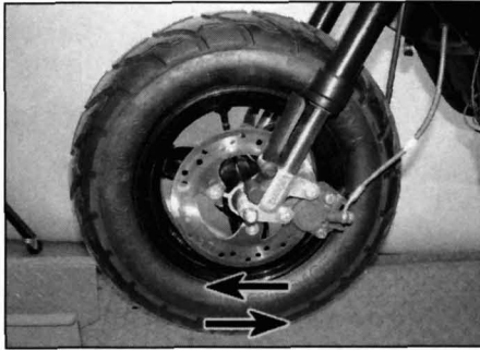
6.4 Freeplay in the bearings can be felt as forwards and backwards movement
