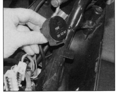
5.7 On Speedfight models, detach the turn signal relay from the handlebars
