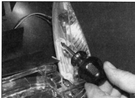
14.9a Undo the screw . . .
