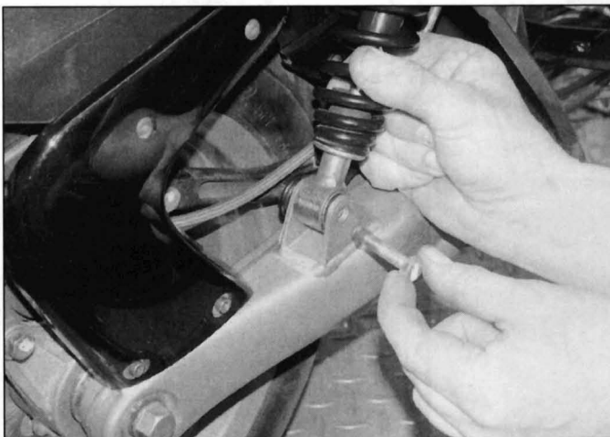
9.27a Thread lock the lower shock mounting bolt . . .
