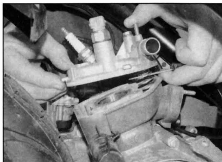
7.18c . . . then hold them in place while the head is installed
