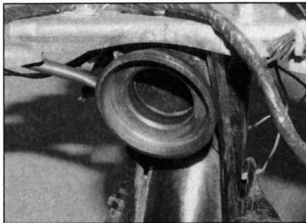
8.3b ... and bottom of the steering head
