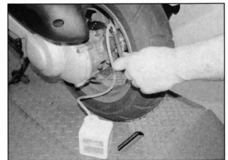
8.5b . . . and attach the hose
