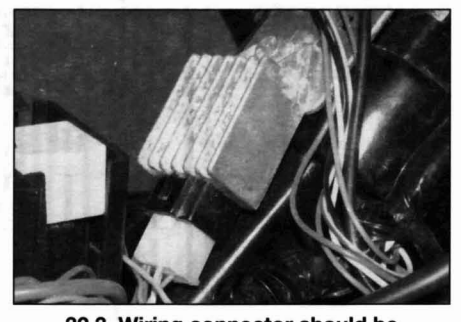
32.3 Wiring connector should be connected to the regulator/rectifier during voltage output checks
