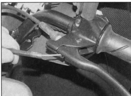
10.4a Pull the cable out of the bracket . . .
