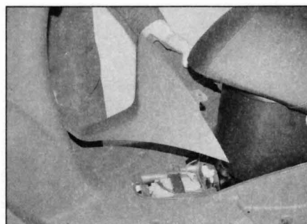
5.4 . . . and lift off the battery panel
