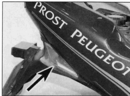
14.1b Retaining screw on rear turn signal lens
