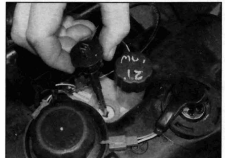
20.8 Withdraw the sensor from the tank
