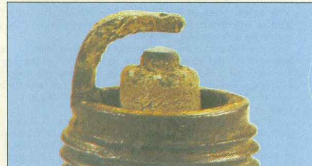
Worn plug – Worn electrodes will cause poor starting in damp or cold weather and will also waste fuel
