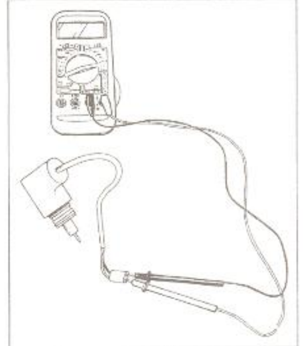
8.18b Automatic choke unit operation check
