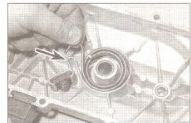
2.10a Fit the return spring, locating its hooked end against the raised section (arrowed)
