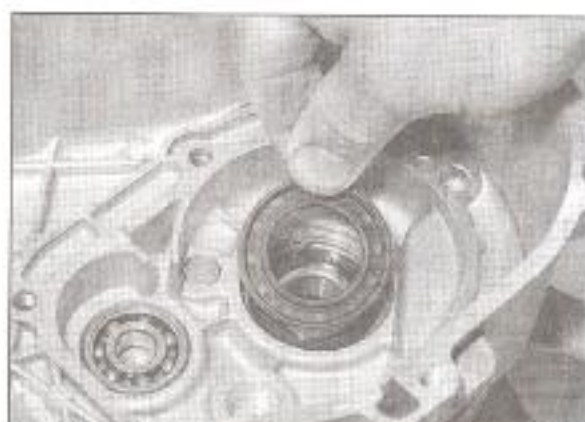
6.13a Lever out the seal . . .
