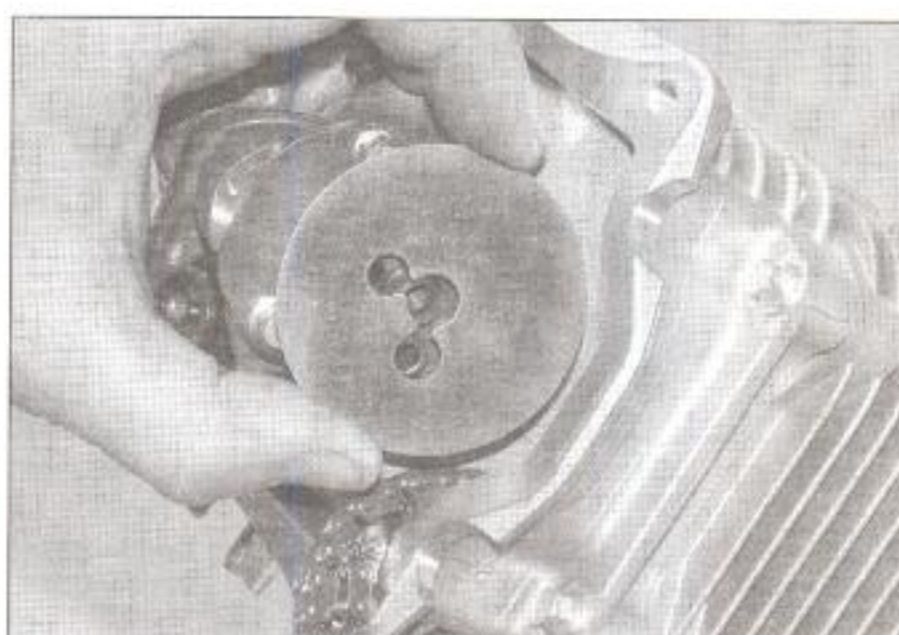
9.23a Install the backing plate ...
