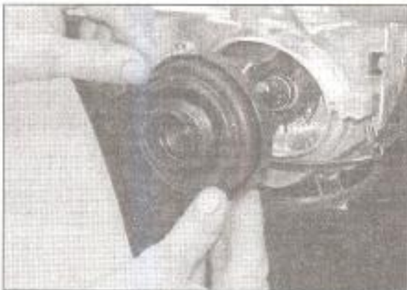
7.3b ... then remove the rubber cover
