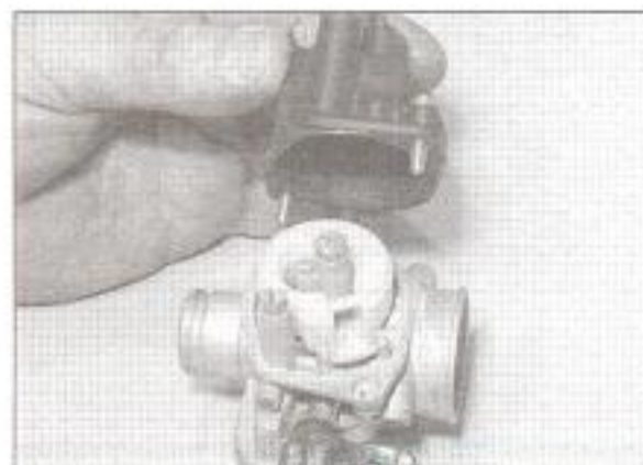
8.4b ... and lift off the chamber
