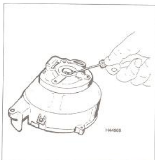
7.22 Lever out the impeller seal
