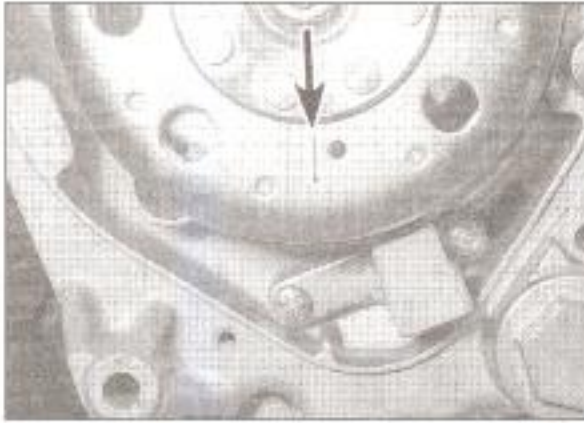
5.4a The timing mark on the rotor (arrowed)
