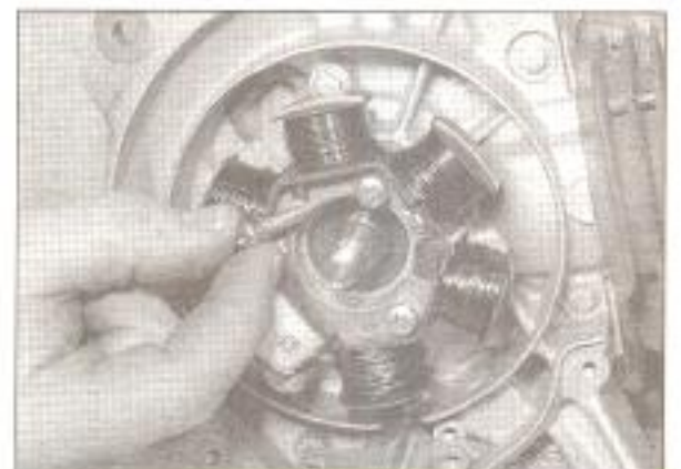
12.6b . . . then install the stator and coil
