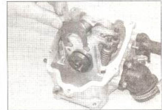
10.5b ... and lift out the plate
