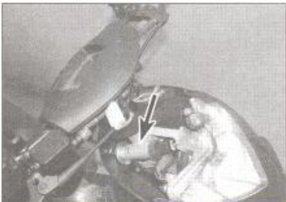
20.2a Location of the ignition (main) switch – Ice shown
