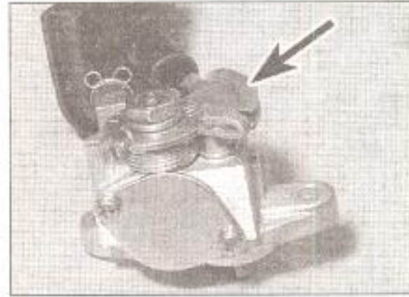
14.5b ... and the cable cam (arrowed) by hand
