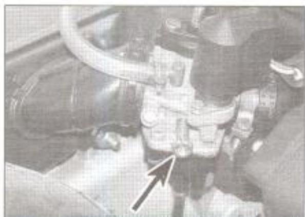
17.3a Idle speed adjuster on slide-type carburettor (arrowed) . . .
