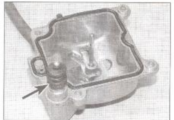
9.7 Unscrew the accelerator pump assembly (arrowed)
