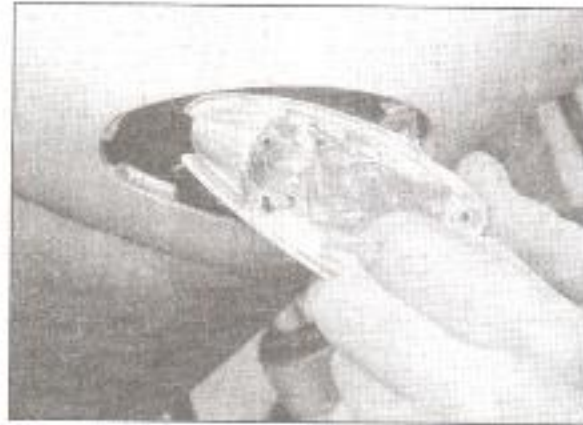
12.1b Twist the bulb cover to remove it
