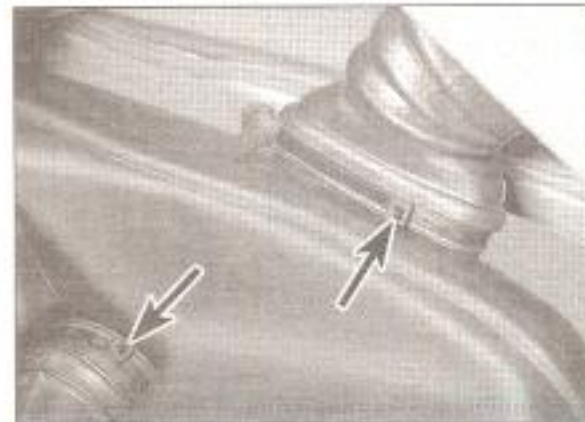
4.1a Release the ties securing the air ducts (arrowed) ...
