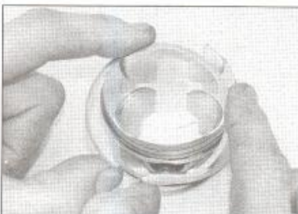
15.3 Removing the piston rings
