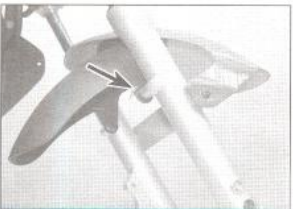
5.28 Note the guide (arrowed) for the speedometer wire
