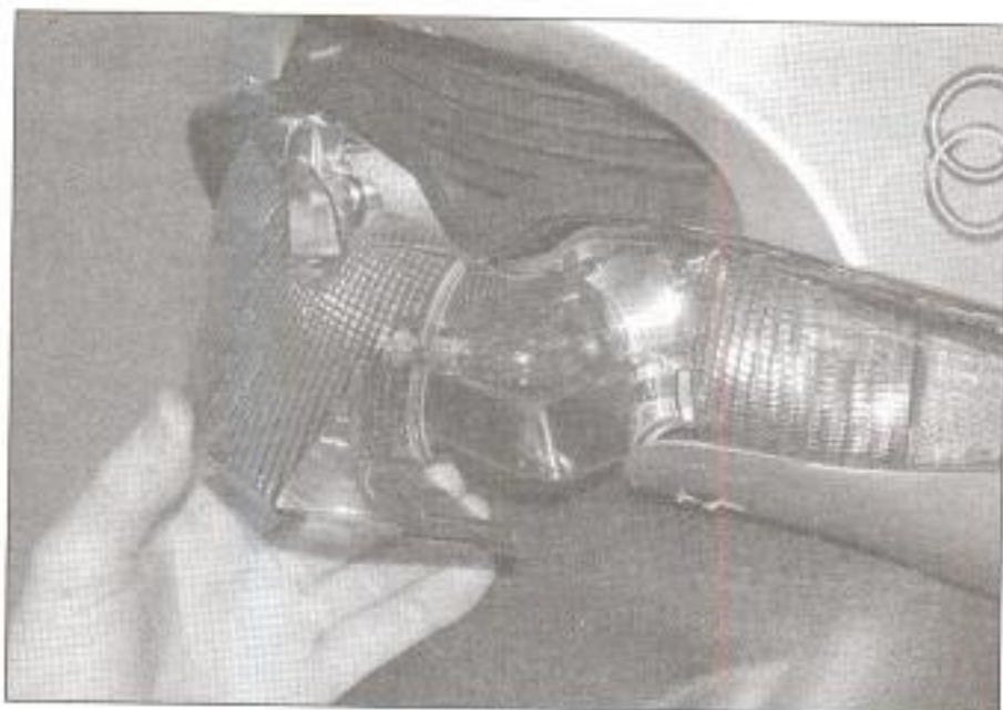
9.1b ... and lift off the lens
