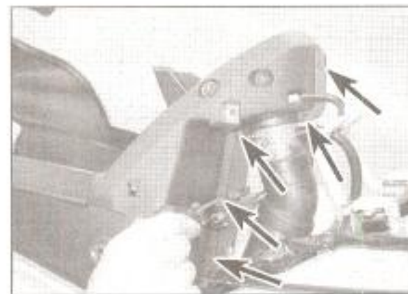
5.16a Remove the five screws (arrowed) ...
