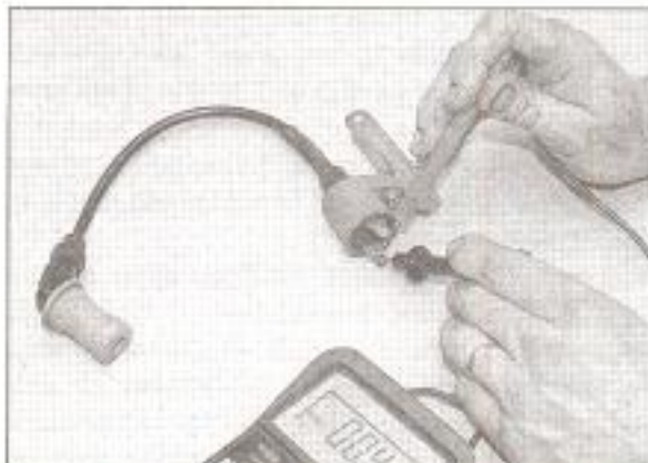
3.9 HT coil primary winding check – Runner VX and DNA 125/180
