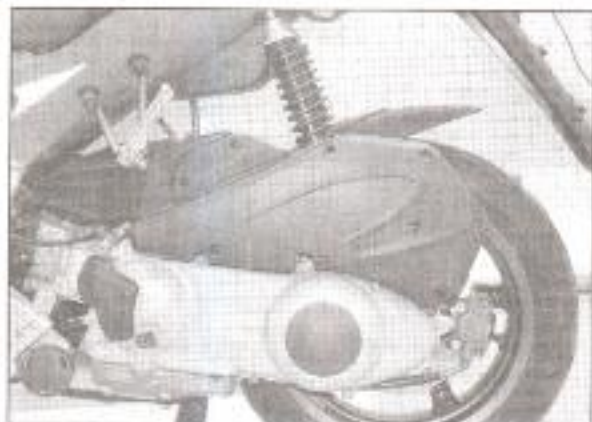
1.2a Remove the screws securing the filter cover – DNA shown
