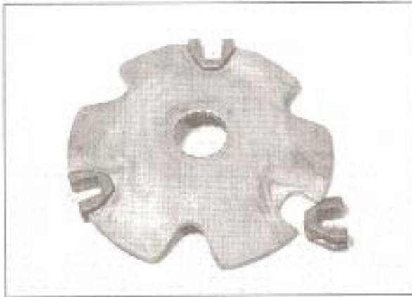
3.14 Check the guide shoes and renew them if necessary
