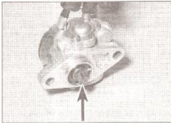
14.5a Rotate the pump drive tab (arrowed) ...
