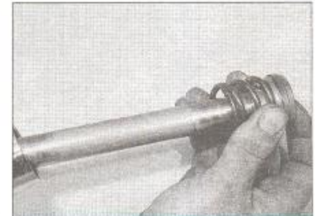
7.51 Withdraw the damper and rebound spring
