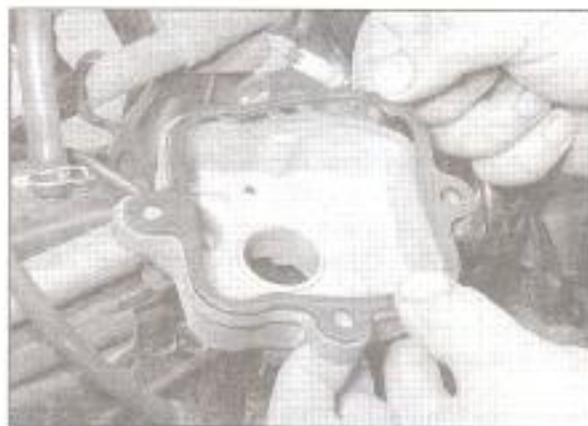
7.19 Check the cover gasket and renew if necessary
