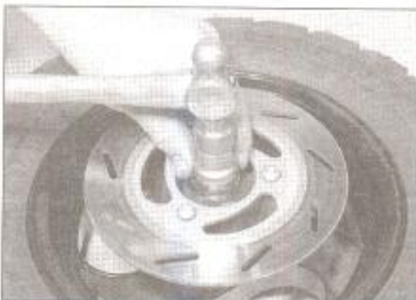
15.11 Using a socket to drive in the bearings
