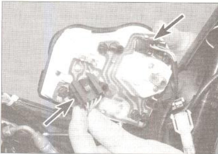
15.4b ... and unclip the wiring connectors (arrowed)
