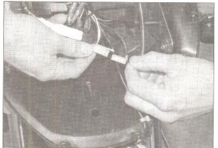
15.6a Disconnect the panel lights wiring connector ...
