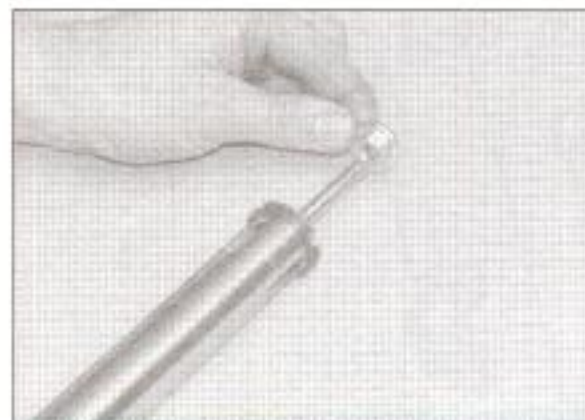
7.20 Thread the inner damper rod nut all the way on
