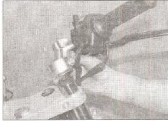
4.14b Lift off the handlebar assembly
