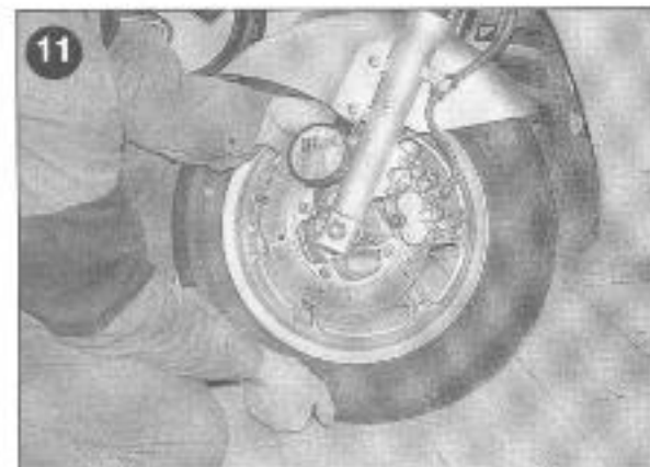
11 Check for wheel bearing play by trying to move the wheel about the axle (spindle)
