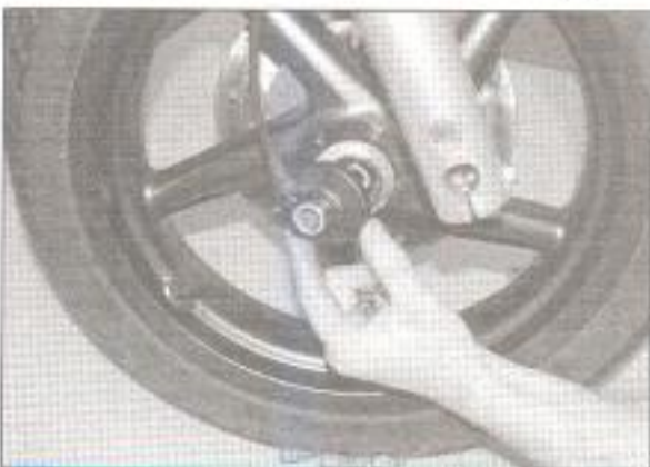
13.5b ... then lift off the speedometer sensor ...
