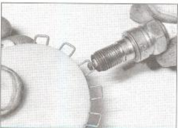
21.6a Using a wire type gauge to measure the spark plug electrode gap
