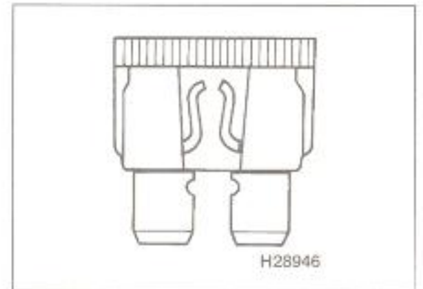
5.2 A blown fuse can be identified by a break in its element
