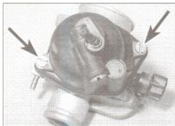
8.4a Undo the screws (arrowed) ...
