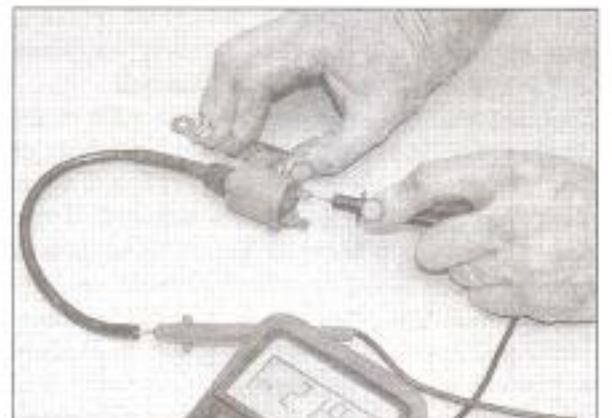
3.10 HT coil secondary winding check – Runner VX125, VXR180/200 and DNA 125/180, plug cap removed
