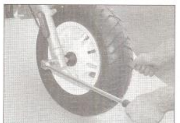
13.6a Counterhold the axle and undo the axle nut
