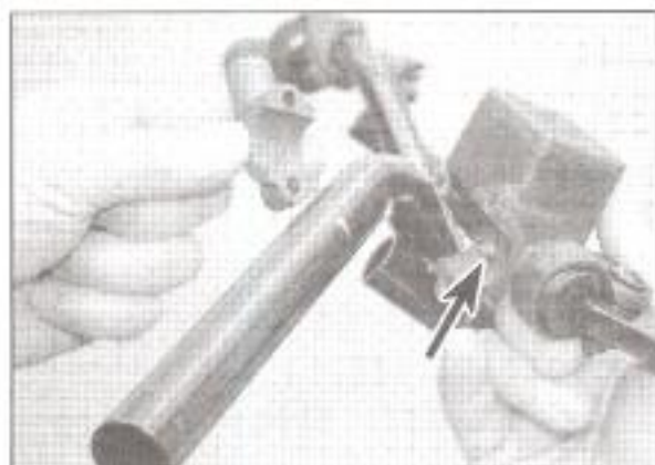
4.7 Note how the pin (arrowed) locates in the hole in the handlebar
