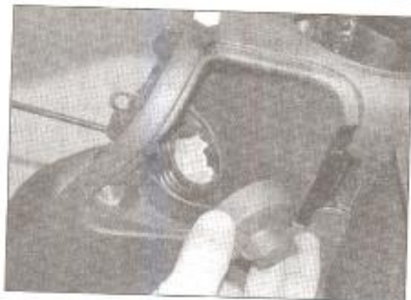
4.35a Remove the fuel filler cap ...
