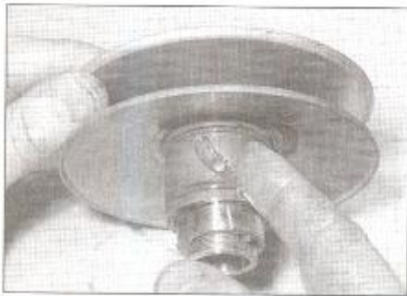
4.16 Apply grease to the slots and around the O-rings
