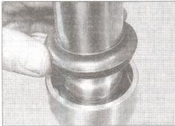
7.61 Install the dust seal
