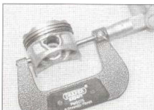
15.8 Measure the piston diameter as described
