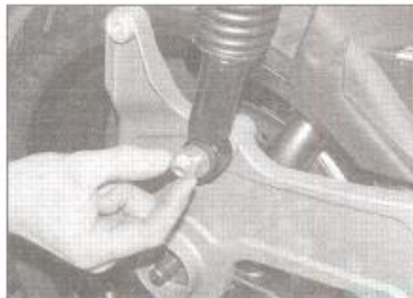
8.5b . . . or remove the nut and washer – twin shock model shown
