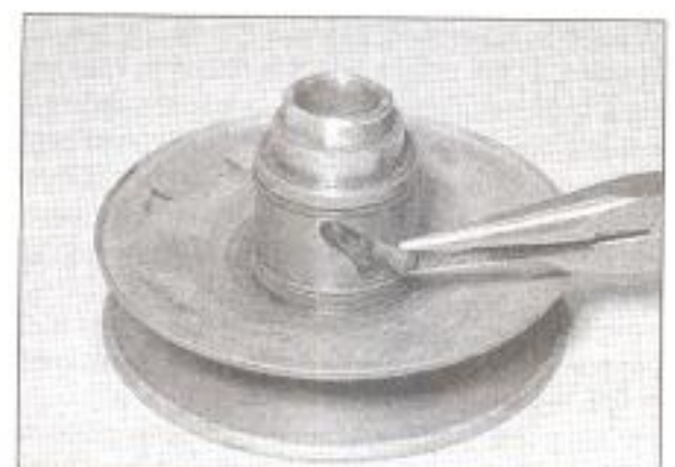
4.7a Withdraw the guide pins ...
