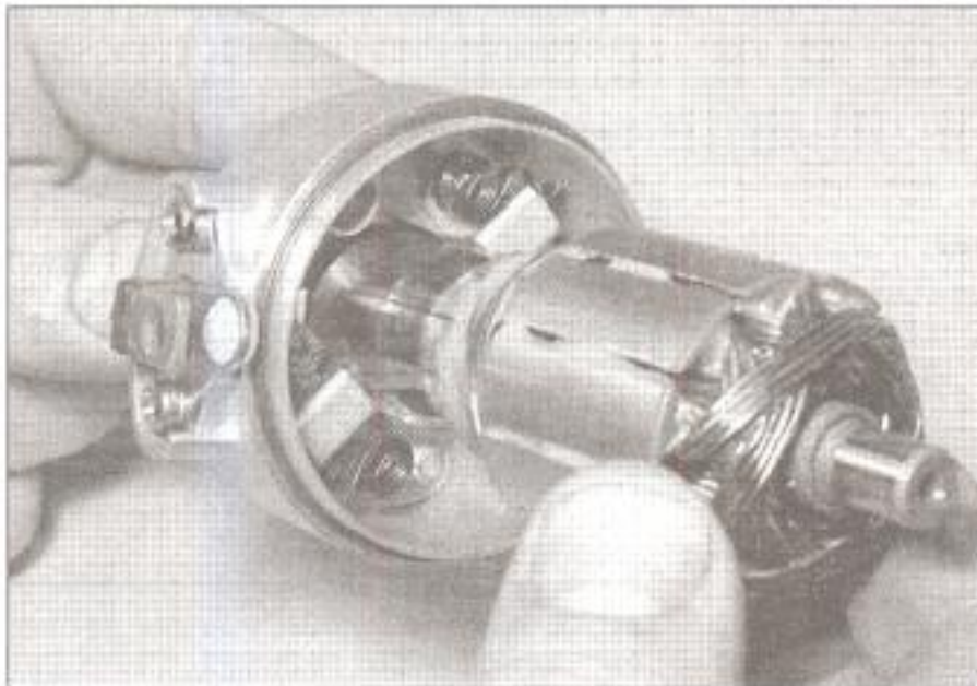
25.4 Withdraw the armature, noting how it fits
