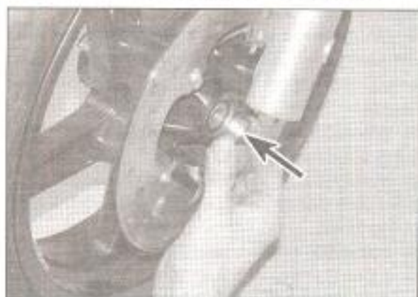
13.5c ... and the left-hand side spacer (arrowed)
