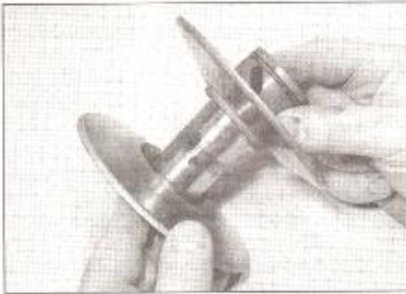
4.7b ... and separate the pulley halves
