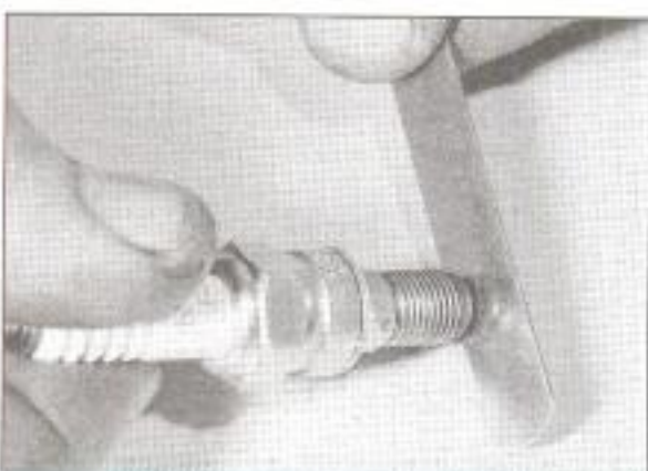
21.6b Using a feeler gauge to measure the spark plug electrode gap
