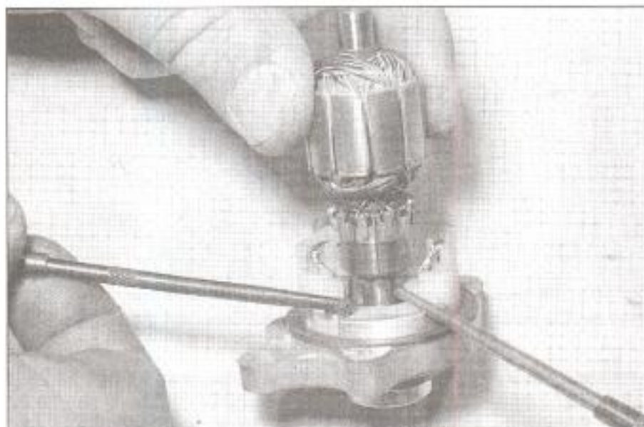
25.14a Hold the brushes back against the springs to allow the armature to be installed
