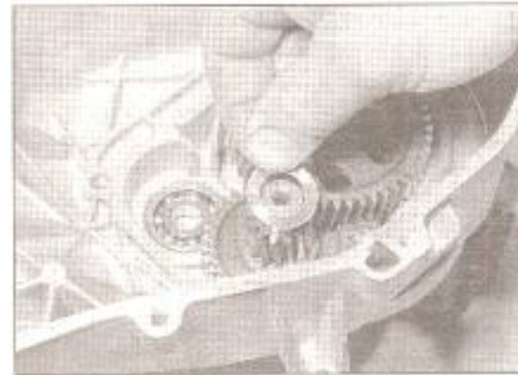
6.4a Remove the outer thrust washer ...
