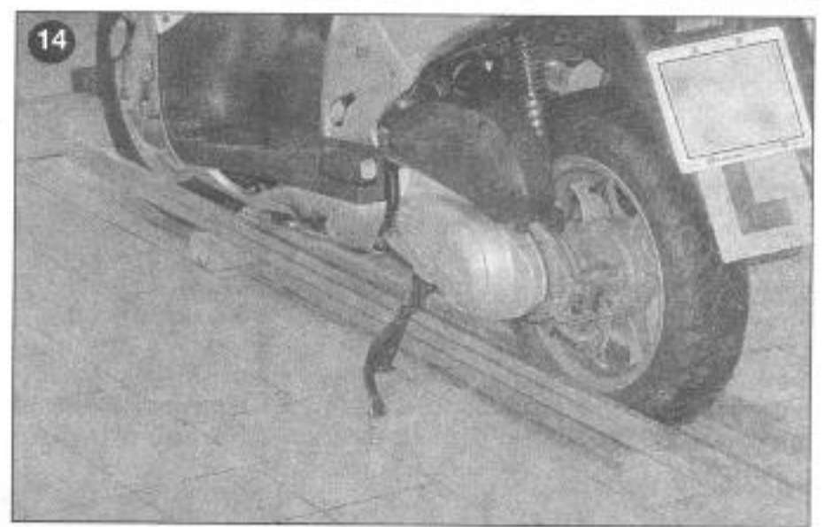
Two straight-edges are used to check wheel alignment
