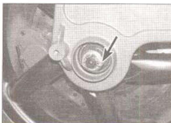
14.18a Remove the split pin (arrowed) ...
