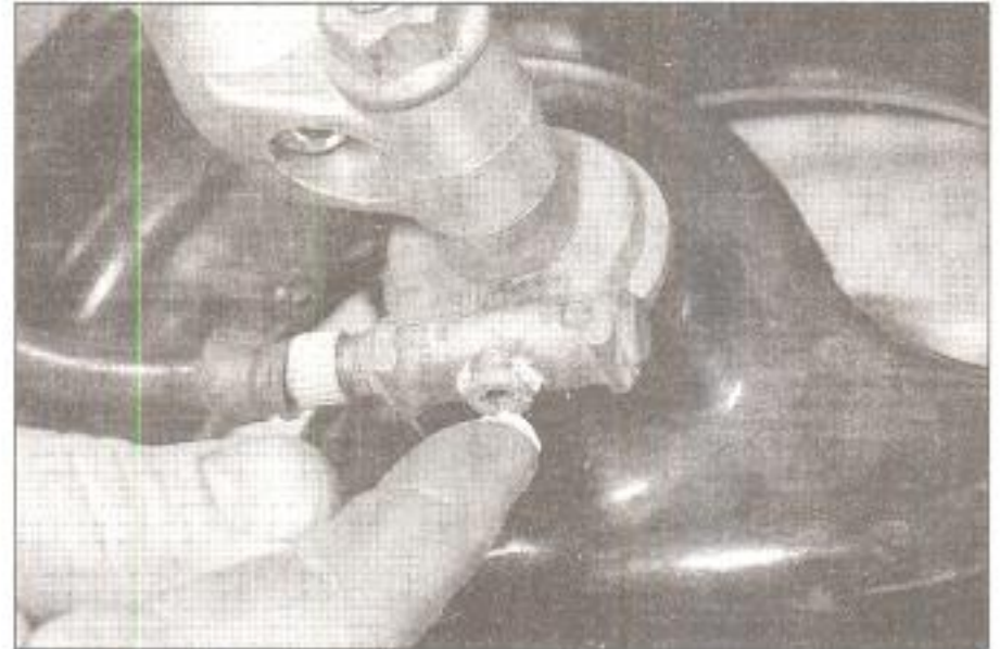
23.4b . . . and press some grease into the housing
