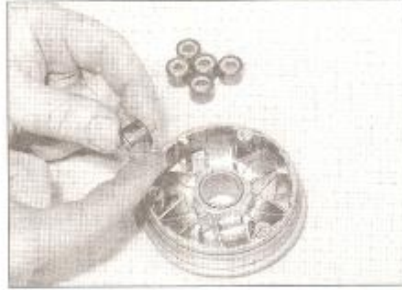
3.15a On early models, grease the rollers and fit them into the housing
