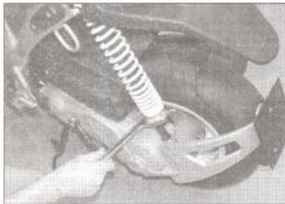
8.1 Adjusting the spring preload – Ice shown
