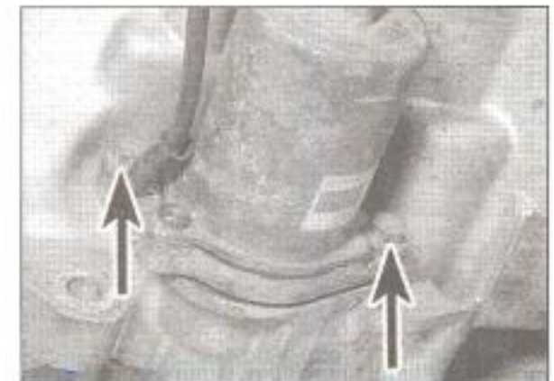
24.2a Remove the two bolts (arrowed), noting the earth cable . . .
