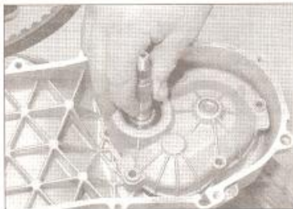
6.3b ... and remove the gearbox cover with the input shaft
