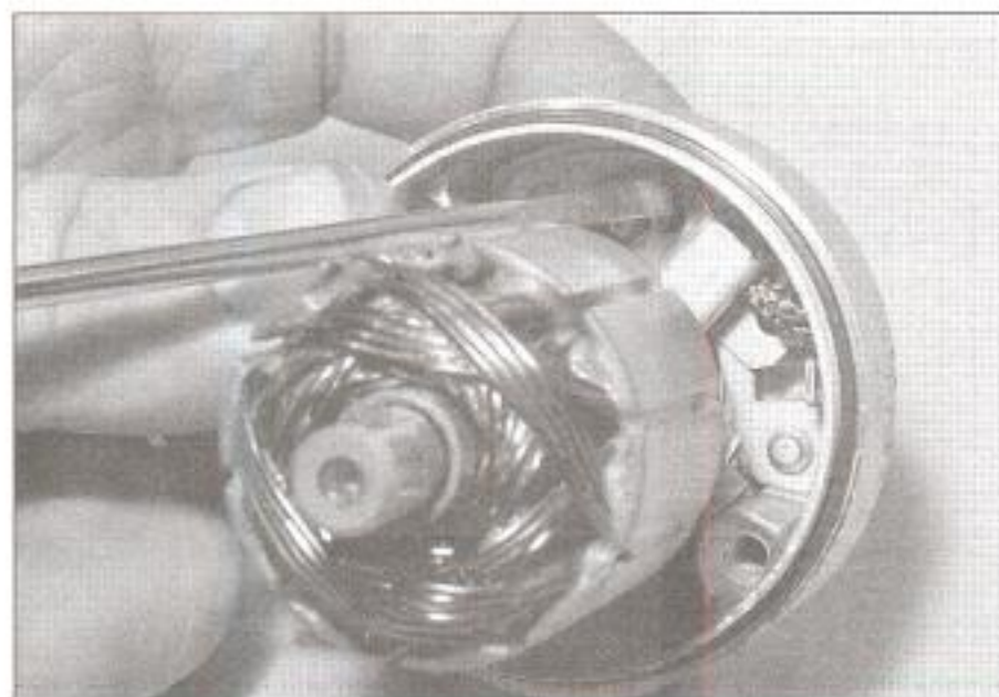
25.14c . . . then locate them back onto the brushes after the armature has been installed
