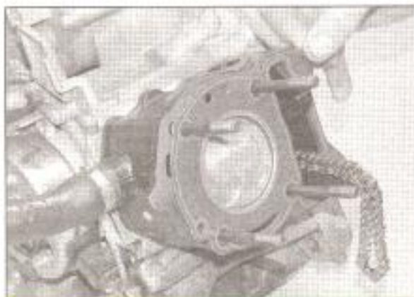
11.10a Remove the head gasket
