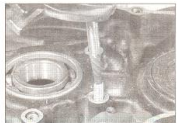
15.13b The extractor is screwed anticlockwise into the broken-off fastener
