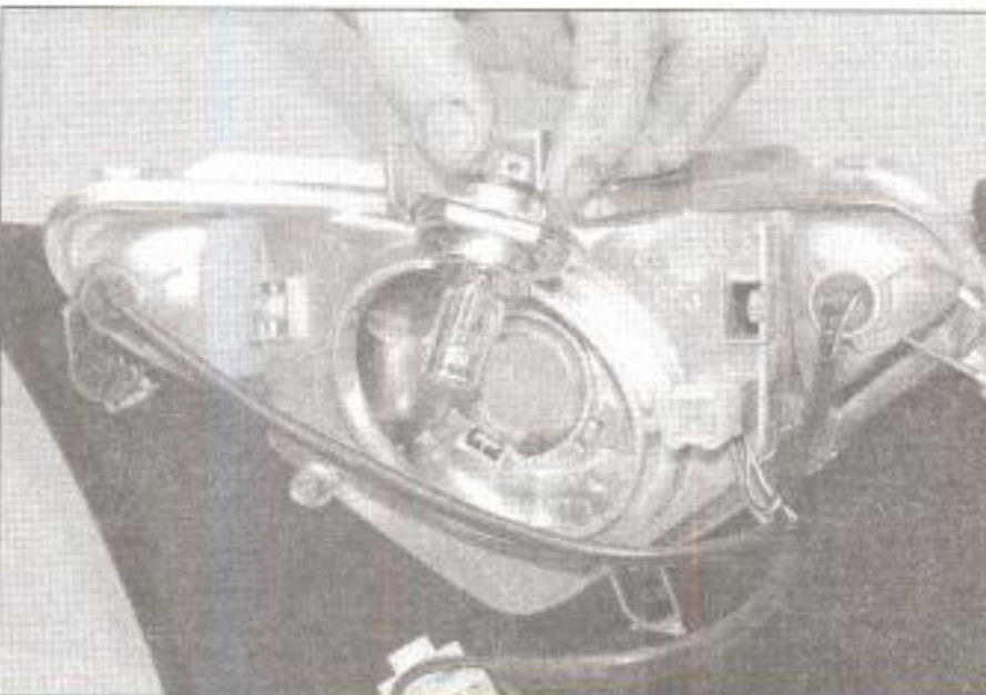
7.5 Handle quartz halogen bulbs by their wire terminals only – do not touch the glass
