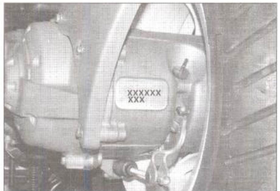
The engine number is stamped into the transmission casing at the back of the rear hub
