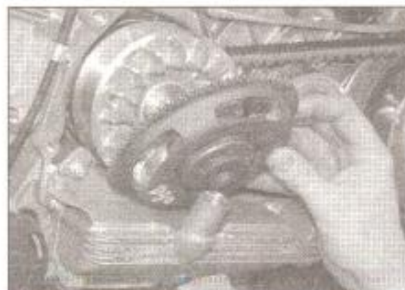
3.8b Slide off the driven gear . . .
