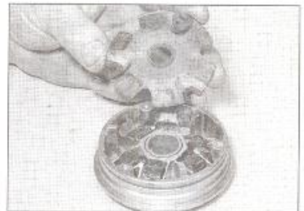
3.11d Lift out the ramp plate ...
