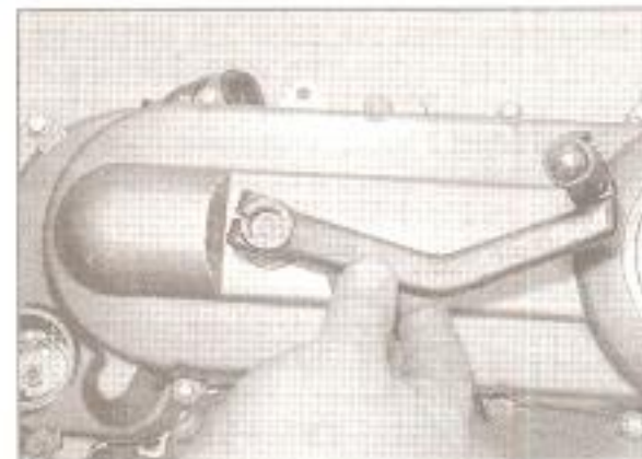
2.8a Unscrew the bolt and remove the kickstart lever
