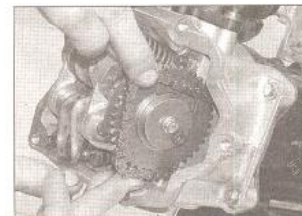
9.13 Lift the cam chain off the sprocket
