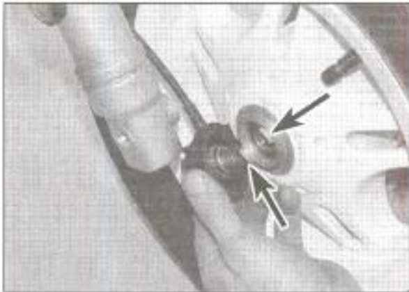
13.6e . . . or sensor – note the drive tabs (arrowed)
