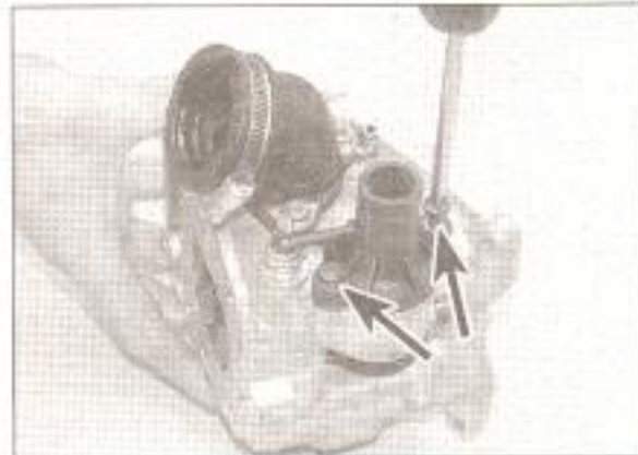
5.3b On four-stroke engines remove the screws (arrowed)
