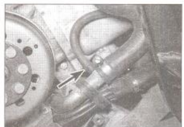
5.2b Detach the hose (arrowed) from its union on the engine
