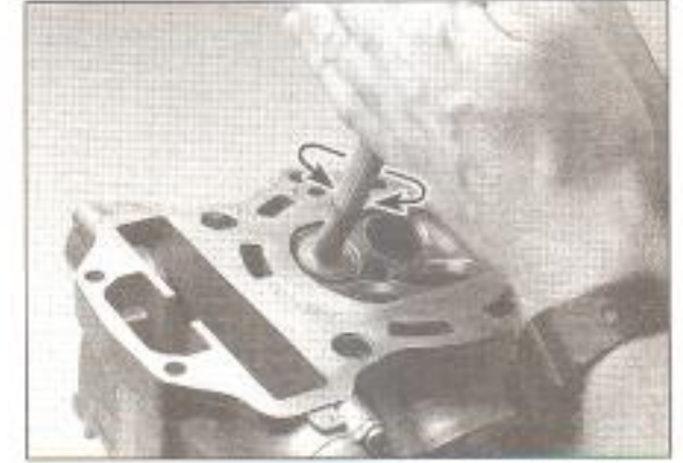
13.20a Rotate the tool back and forth between the palms of your hands
