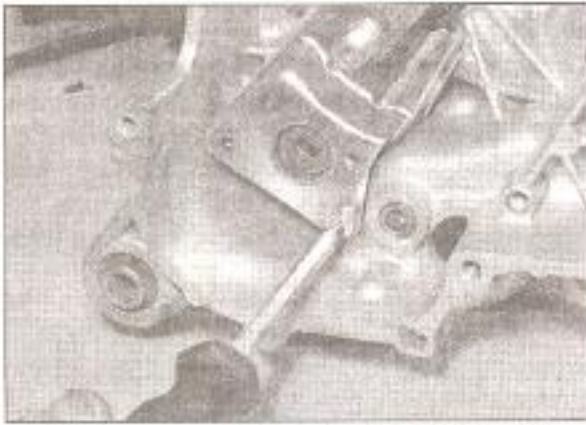
14.4a Remove the screw securing the guard plate ...
