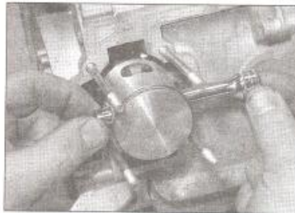
9.3b ... and push out the piston pin, using a socket extension if required
