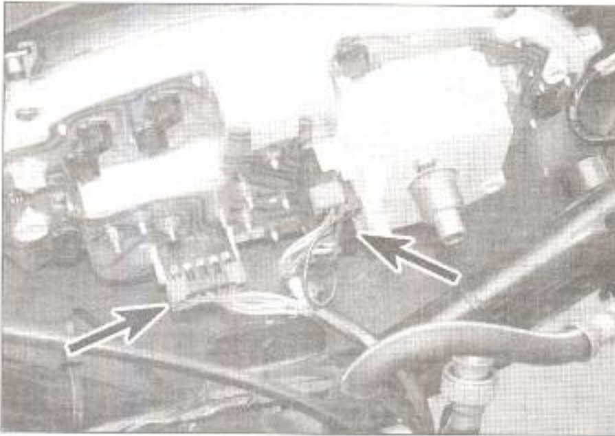
15.3 Instrument cluster wiring connectors (arrowed) on Runner models
