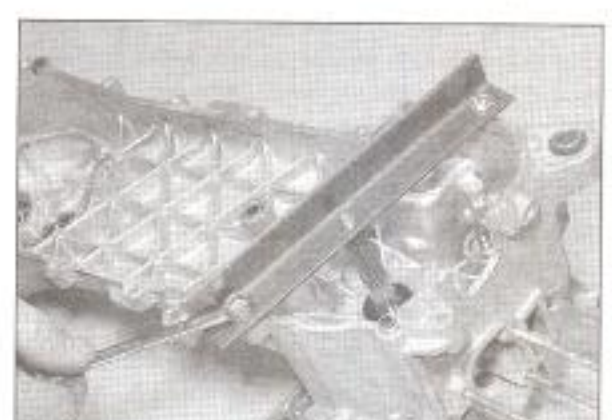
15.5 Pressing the crankshaft out of the left-hand crankcase half
