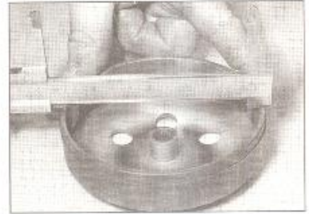
4.10 Measure the drum diameter as described
