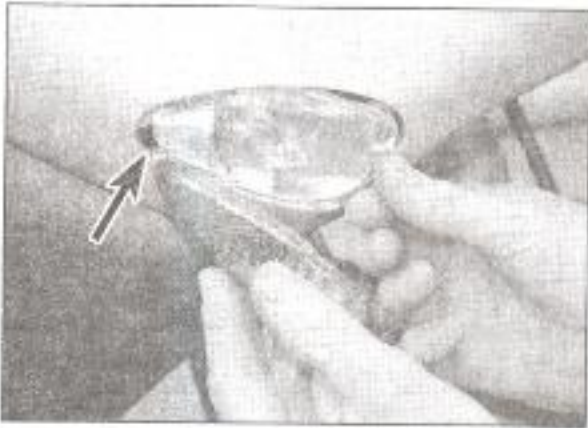
12.1a Note how the tab (arrowed) locates in the panel
