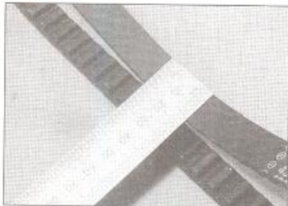
5.2 Measure the width of the belt to determine wear
