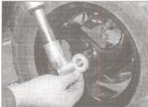
13.6f Remove the thrust washer where fitted
