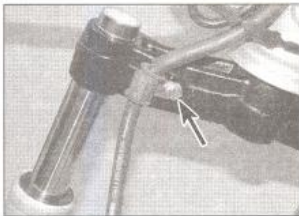
5.1 Detach the brake hose clip from the steering stem
