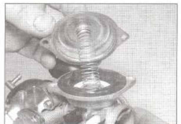
9.32 Locate the cover onto the spring and fit it onto the carburettor
