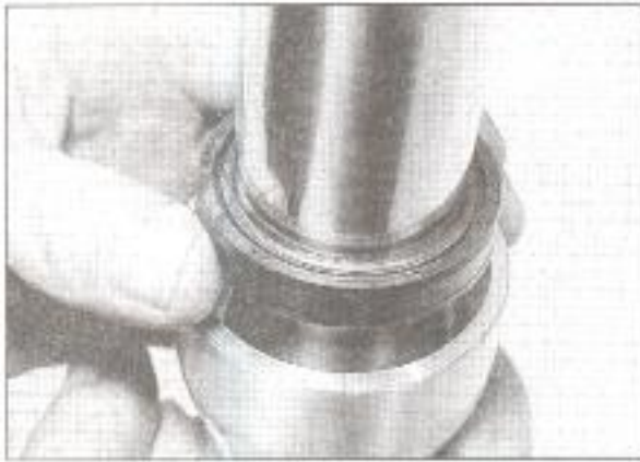
7.60a Install the oil seal with markings facing up
