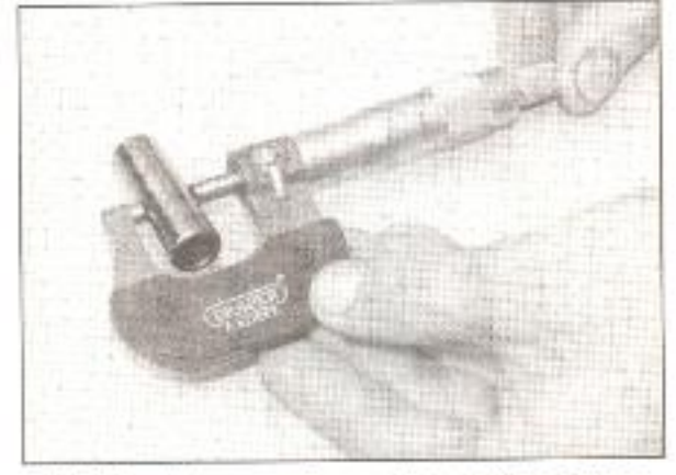
15.10a Measure the centre of the piston pin ...
