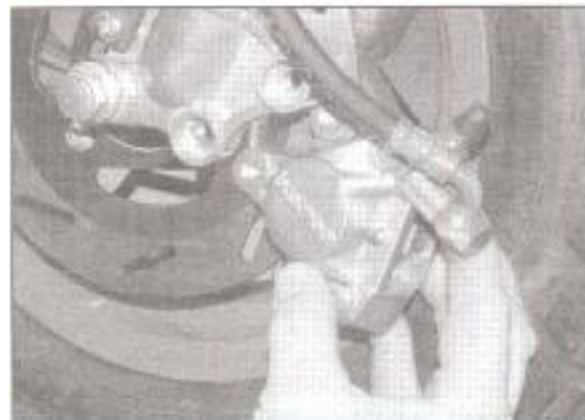
3.3b . . . and slide the caliper off the disc
