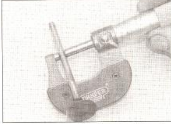
13.13 Measuring the valve stem diameter with a micrometer
