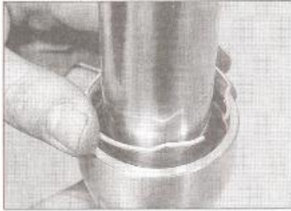
7.60b Install the oil seal retaining clip
