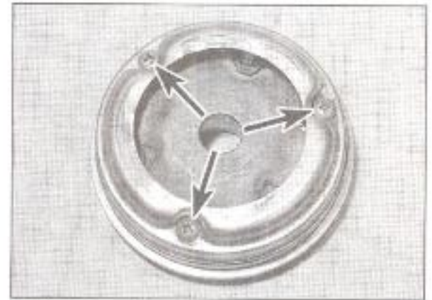
3.11a On early models remove the screws (arrowed) ...
