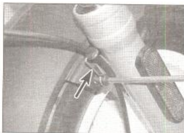
6.49 Note the guide (arrowed) for the speedometer wire
