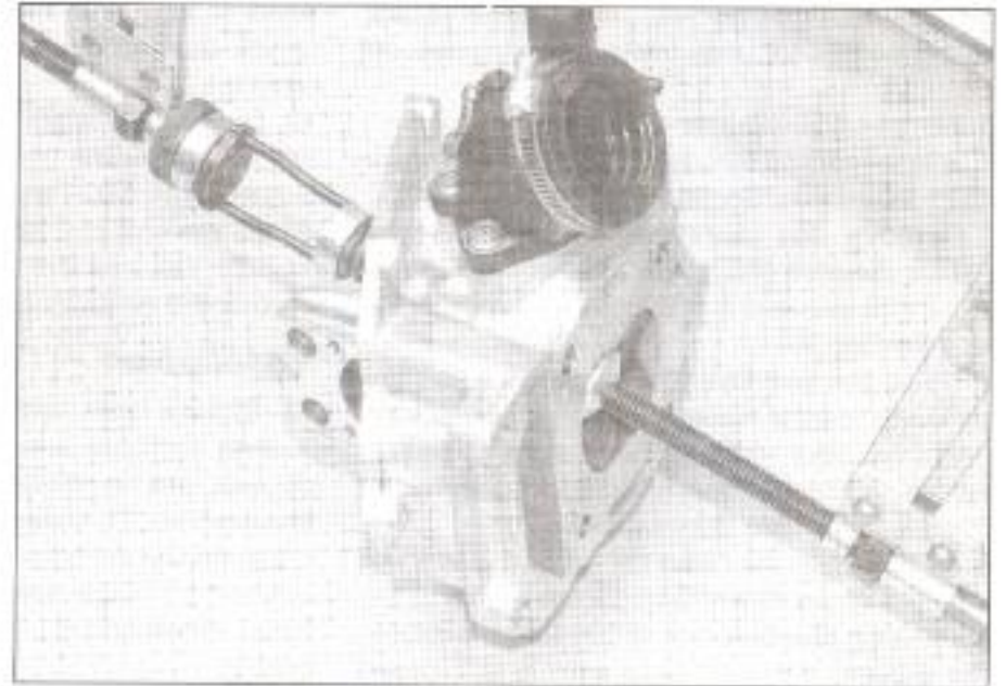
13.5a Compress the valve spring ...
