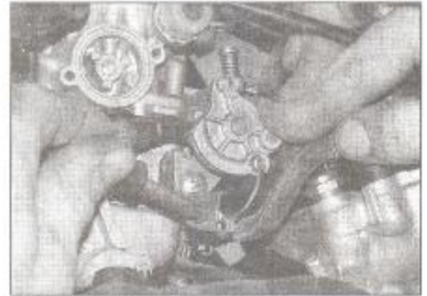
12.13b ... then detach the inner cable end from the cam
