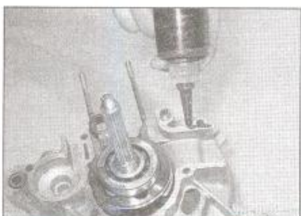
15.20 Apply sealant to the crankcase mating surface
