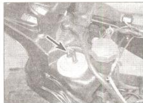
18.1b Fuel level sensor wiring connector – SKP/Stalker shown
