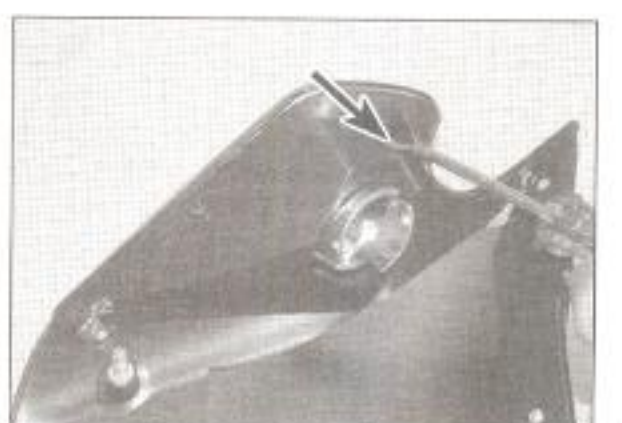
13.2c Remove the screw (arrowed) . . .
