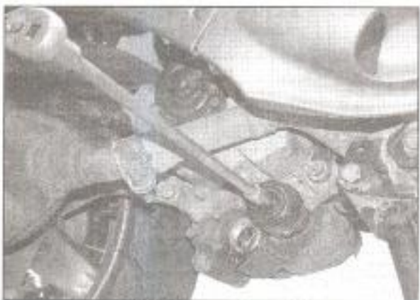
12.5a Unscrew the oil filter
