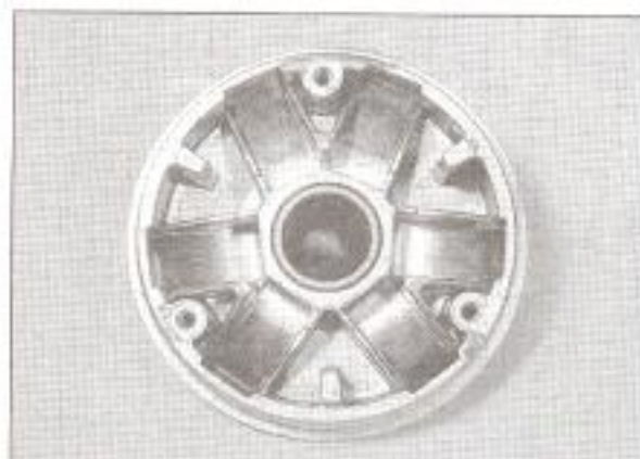
3.12a Check the ramps for wear
