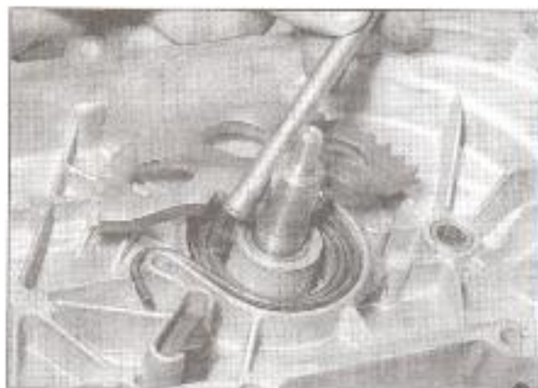
2.10c . . . then locate the steel rod onto the spring end and against the pinion . . .
