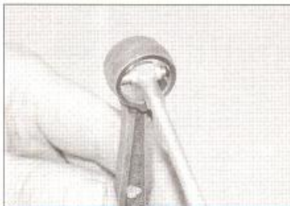
9.16 Measuring the internal diameter of the connecting rod small-end
