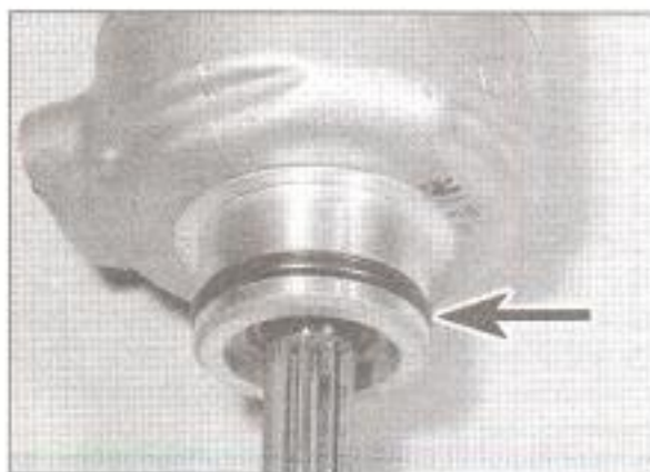
24.7 Fit a new O-ring if applicable
