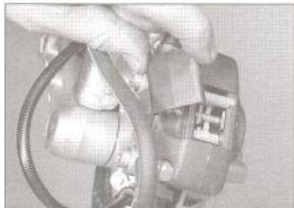
2.1 Remove the cover from the caliper
