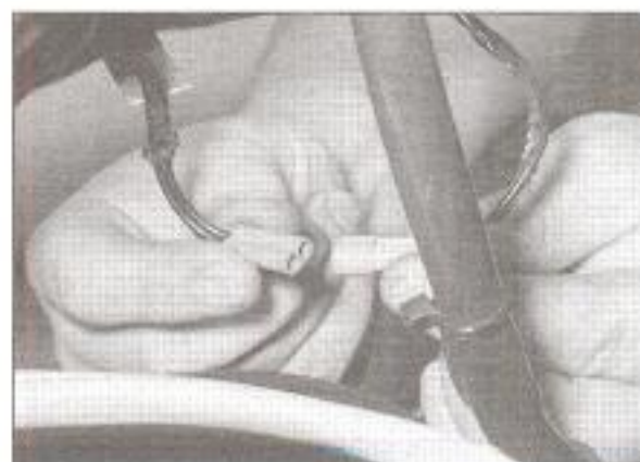
7.2 Disconnect the choke wiring at the connector
