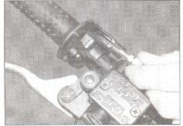
12.5c Pull the cable out of the elbow ...
