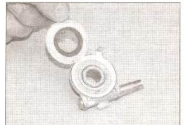
23.6 Lubricate the speedometer drive gear with clean grease
