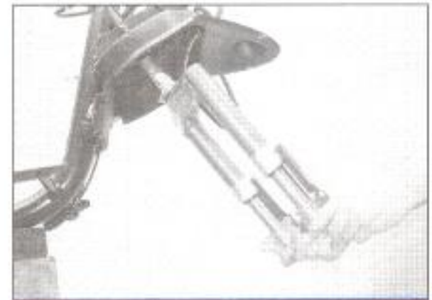
5.6 Lower the steering stem out of the frame
