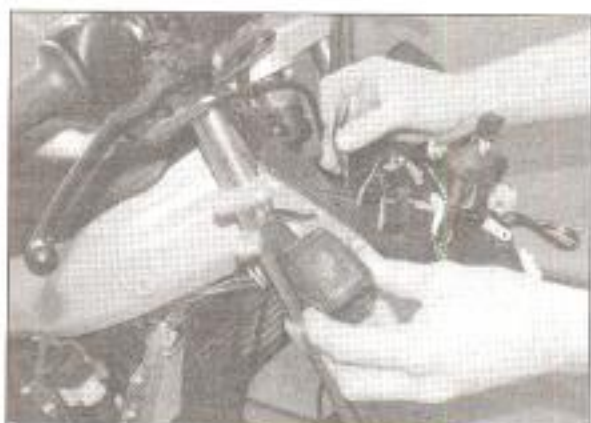
13.2b . . . then feed the wiring through the hole in the headlight bracket
