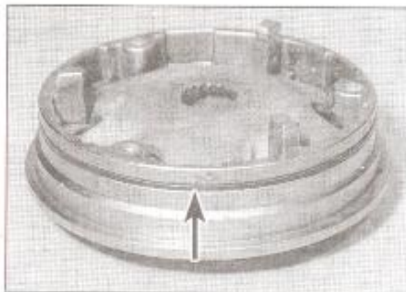
3.11c Discard the O-ring (arrowed)
