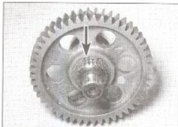
6.11 Remove the circlip (arrowed) and slide the pinion off the output shaft
