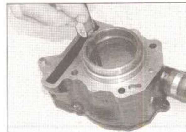
16.2 Measuring piston ring installed end gap
