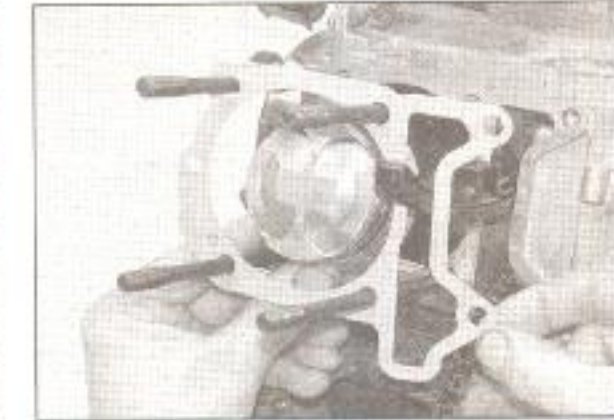
14.20 Fit a new cylinder base gasket onto the crankcase
