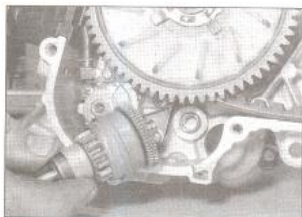
13.2 Remove the starter pinion assembly, noting how it fits
