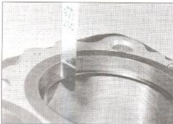
10.2 Measuring piston ring installed end gap
