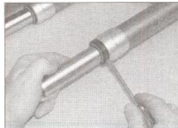
7.2c Lever out the seal
