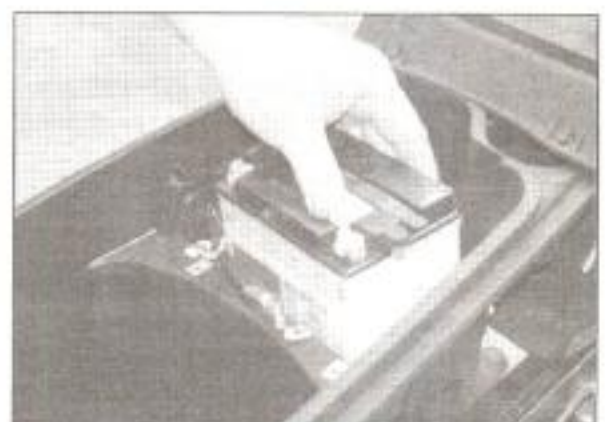
3.2b . . . and lift out the battery
