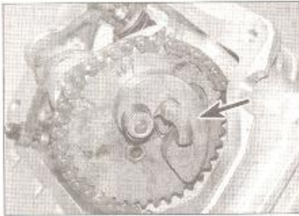
9.24 Install the bob weight (arrowed)
