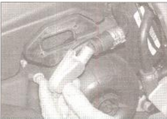
20.2c . . . and pull off the reed valve housing
