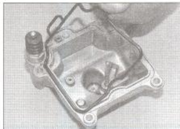
9.29 Ensure the float chamber gasket is correctly located
