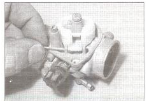
8.5 Withdraw the float pin
