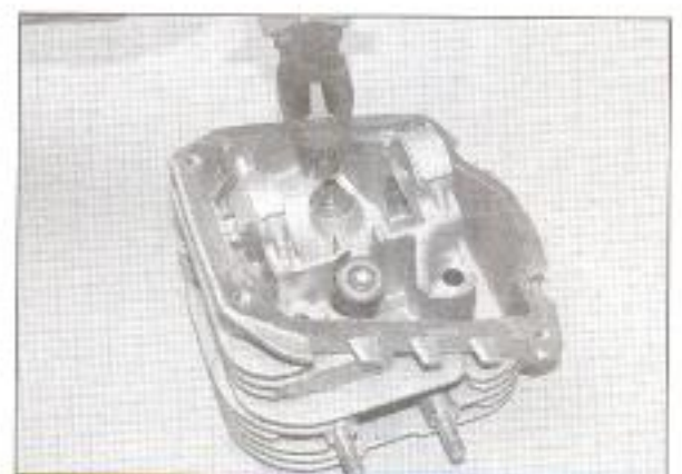
13.5f Pull the stem seal off with pliers
