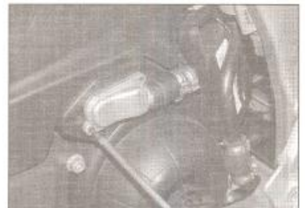
20.2b . . . then remove the housing screws . . .
