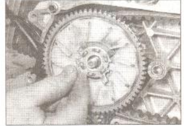
3.6a Remove the mating plate . . .
