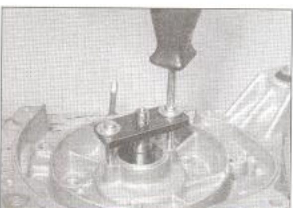
15.4 Drawing the right-hand crankcase half off the crankshaft
