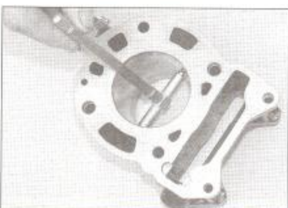
14.8a Measure the cylinder bore with a telescoping gauge as described
