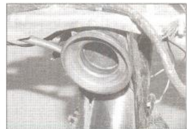
6.3 Check the outer races in the steering head
