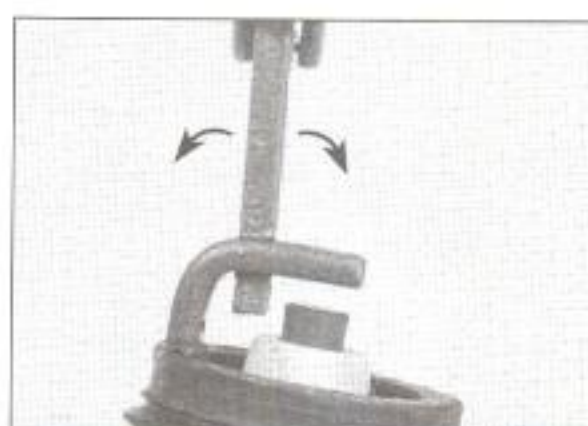
21.6c Adjust the electrode gap by bending the side electrode only
