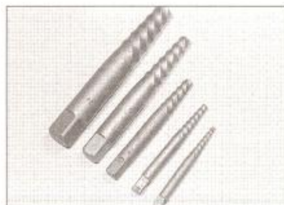
15.13a A set of screw extractors is a useful addition to the workshop
