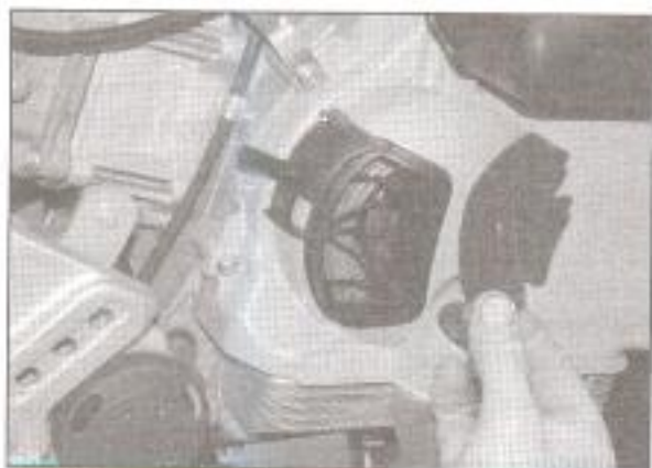
1.8b . . . and lift out the filter element
