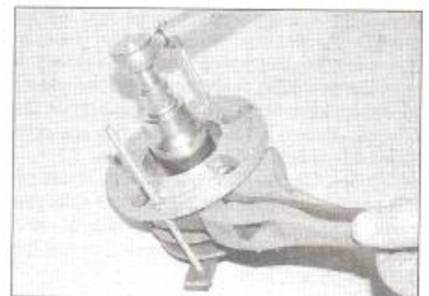
4.5 Hold the clutch with a strap wrench and unscrew the nut
