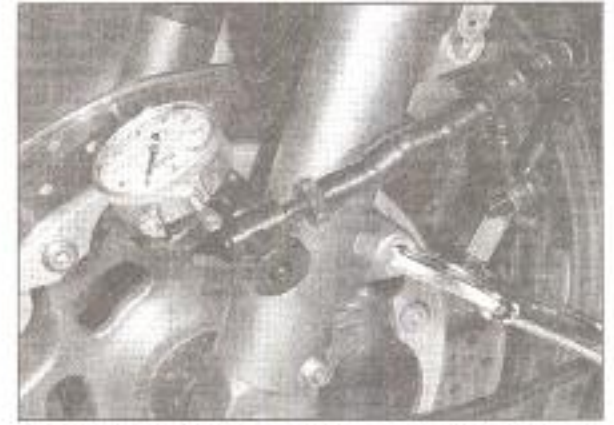
4.2 Set-up for checking brake disc runout
