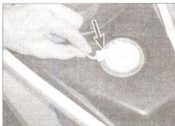
18.1a Fuel level sensor wiring connector – Ice shown
