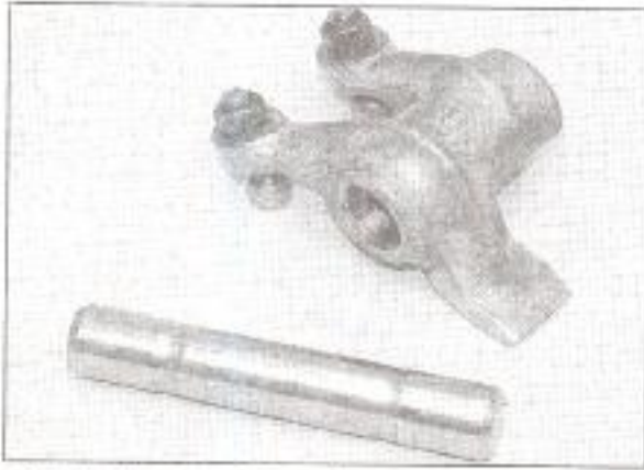
10.7b Keep each rocker arm and its shaft together
