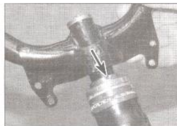
4.9c Note how the peg (arrowed) locates in the slot
