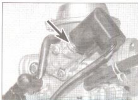
9.34 Secure the choke unit with the clamp (arrowed)
