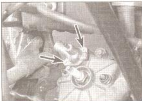
5.3a On two-stroke engines remove the screws (arrowed)
