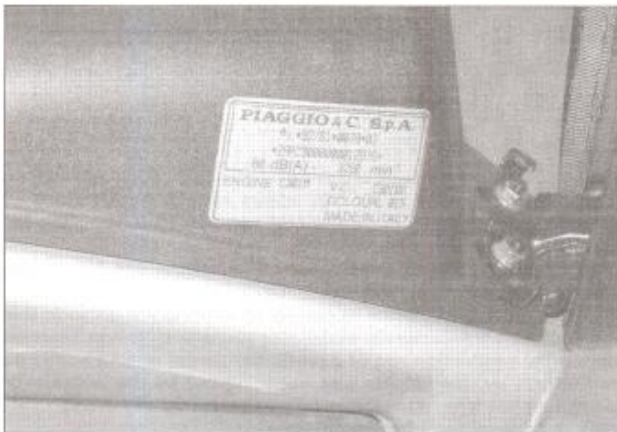
The frame number also appears on the identification plate
