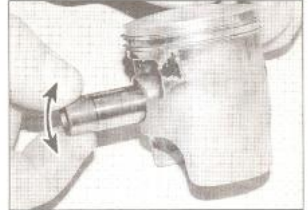
9.15 Checking for freeplay between the piston and the piston pin
