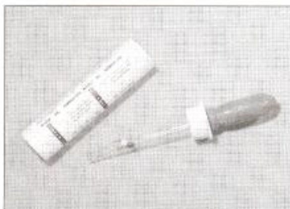
9.7 An antifreeze hydrometer is required to check coolant strength
