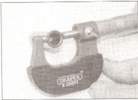
15.9a Measure both ends of the piston pin ...
