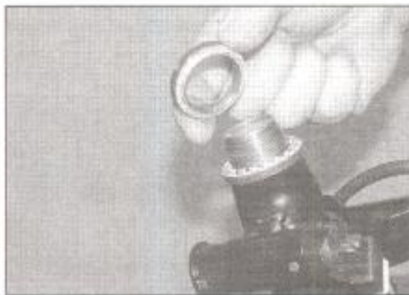
5.5a Remove the bearing adjuster nut – SKP/Stalker shown
