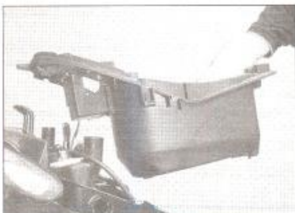
7.17 ... and lift out the storage compartment
