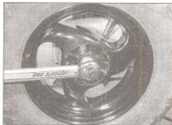
14.6 Tighten the nut to the specified torque
