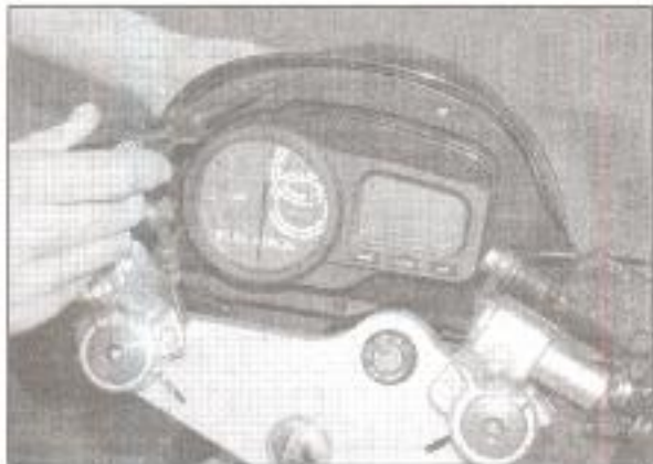
5.19a Remove the screws from around the edge of the fairing . . .
