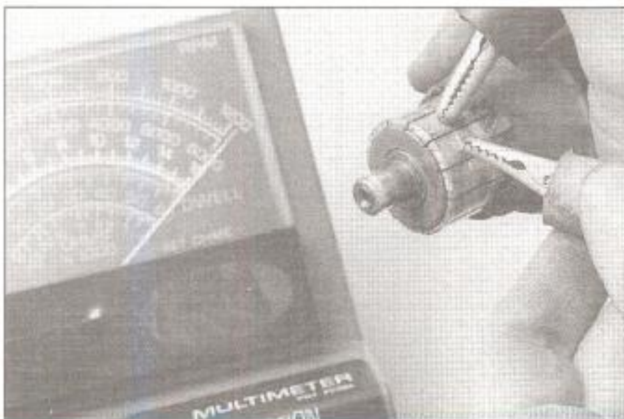
25.8a Continuity should exist between the commutator bars
