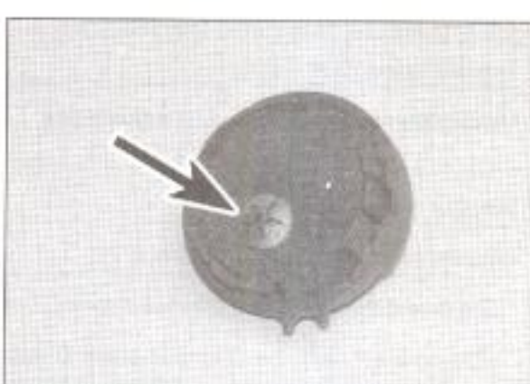
1.8d The filter element is secured by a small clip (arrowed)
