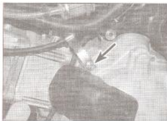
5.8a Free the throttle cable clip (arrowed) . . .
