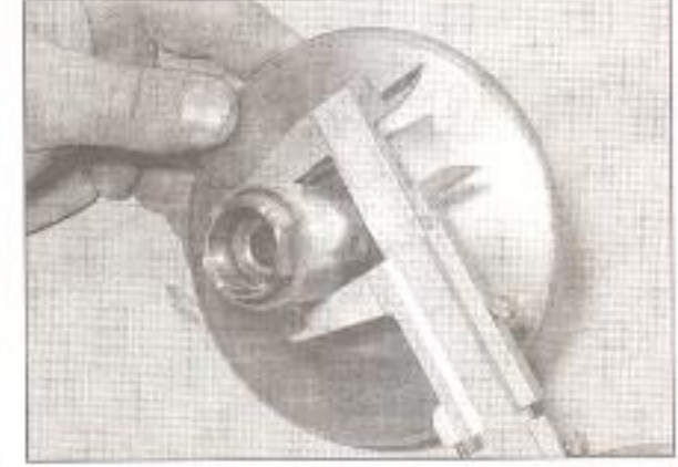
4.13a Measure the diameter of the inner pulley shaft ...
