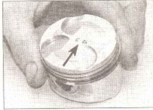
14.8c Piston size code (arrowed) stamped into the crown
