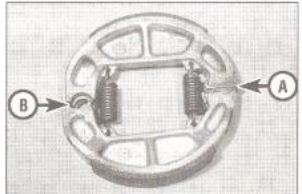
9.10 Fit the springs and locate the flat ends (A) against the cam and the rounded ends (B) against the pivot
