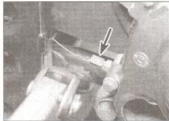
12.8b ... and draw the cable out of the adjuster
