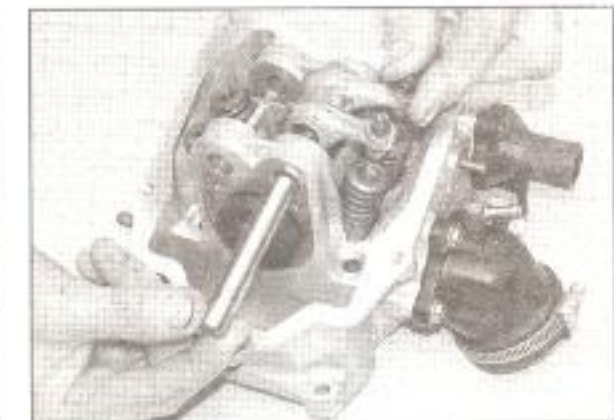
10.7a Withdraw the rocker shafts
