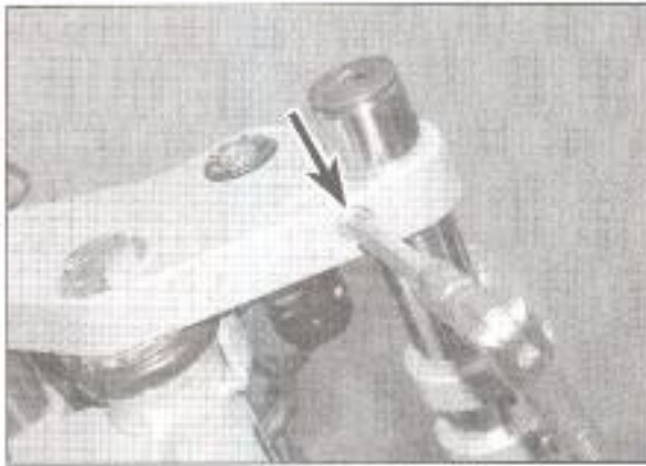
5.3a Loosen the upper fork leg clamp bolts
