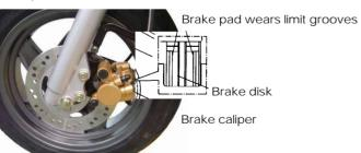
Check the brake from behind the brake caliper. The brake pad must be replaced with new lining when the brake pad wear limit reaches the brake disk.
