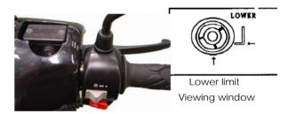
Park the motorcycle on a level ground, and check if fluid level is under the "LOWER" mark. Recommended Brake Fluid: CASTROL SUPER DISK BRAKE FLUID DOT 4.
