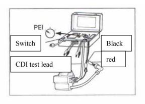
Note the spark in the spark gap window. It should be strong and continuous, not intermittent, acrossa preset 8mm(0.32in) gap. Allow the spark to jump the test gap for at least five minutes continuously. To insure proper operation under the temperature of actual riding.
