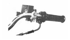
Remove the brake lever and brake switch.
