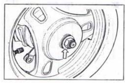
• remove brake shoe and rear axle 6.
