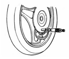
With the disc mounted on the wheel, check the dids for face runout with a dial gauge as shown.
