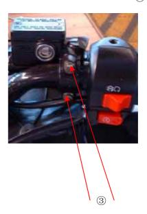
3. Disconnect throttle cable  $\ensuremath{\mathfrak{I}}$  and oil pump cable  $\ensuremath{\mathfrak{I}}$
