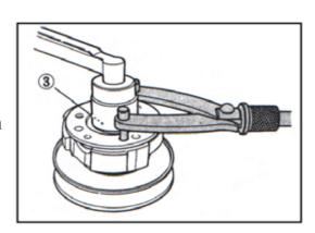
• insert the V-belt between the driven faces as deep inside possible while pulling the movable driven face all the way outside to provide the maximum ble clearance.
