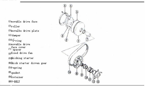
Apply grease to all the sliding and rolling surfaces for six roller weights. For each weight, approximately 1.5g of grease should be used.
