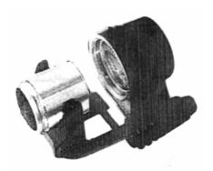
Inspect each rubber part for damage and wear.
