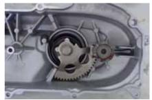
• Remove starting driven ratchet wheel by removing the nuts.
