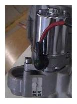
• Remove the clutch housing with the special tool. (Peg key)
