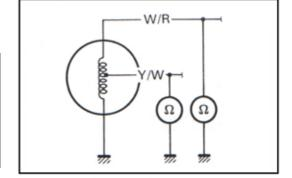
Use procket tester to measure the resistance between the lead wire and ground. If the resistance checked is not correct, replace the coil.
