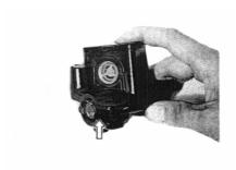
Remove the circlip with the special tool.
