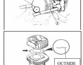
tighten the cylinder head nut to the specification.
