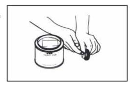
• Install oil seal into crankcase carefully with special tool.
