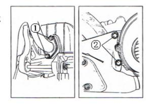
• lubricate brake cam shaft with GENERIC grease.
