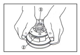
• tighten the nut③ to the specified torque with the special tool.
