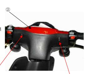
2. Remove master cylinder by removing the bolt  $\ensuremath{\mathfrak{G}}$ ;
