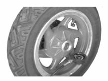
When installing this speedometer gear box, align the two driving pawls with the two recesses of the wheel hub. Tighten the nut with special tool.
