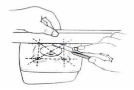
If the largest reading at any portion of the staightedge excees the limit, rework the surface by rubbing it against emery paper laid flat on the surface plate in a lapping manner. The surface must ge smooth and perfectly falt in order to secure a tight join: a leaky joint can be the cause of reduced power output and increased fuel consumption.
