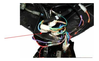
6. Remove handle cover by unscrewing bolt  $\, \, \textcircled{6} \,$
