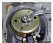
• remove magneto rotor and half circle key with special tools.
