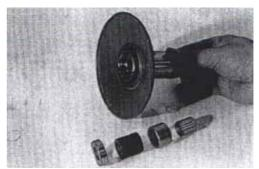
Remove the oil seal from the gearcase cover with the speical tool.
