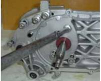
• screw oil drain nut○,¹¹ tightening torque: 4-7 N.m (0.4-0.7kg-m,3.0-5.0 Ib-ft)
