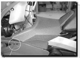
• After extracting the 6 side screws and the central one (Allen M3 5x12) from the tank cover, lift the front of this removing the 2 lugs, and then remove the back part as in the image.
