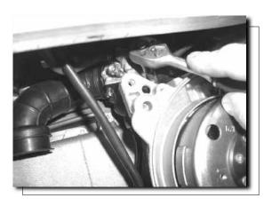
• Disconnect the choke cable, petrol pipe and air inlet pipe from the carburettor. Next, turn it and extract the top cover.
