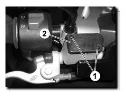
Purge the air completely from the master cylinder using this procedure.
