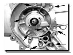
Install the special plate on the flywheel-side half crankcase and proceed by splitting the two halves.
