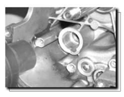
Using the air heater, warm up the water pump bearing housing, without directing the air flux directly aginst the oil seal
