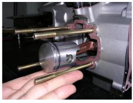
Install the cylinder gasket. Coat the cylinder and piston ring with the engine oil. Install the cylinder.
