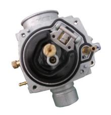
Remove the main jet, slow jet, needle seat & air screw.
