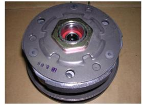
Fix the driven pulley in a compressor. Remove the special nut (28mm). Release the compressor. Remove the driven plat assy.
