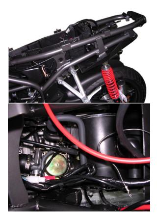
Disconnect the fuel & the vacuum tube. Disconnect the spark plug cap. Disconnect the rear brake cable.
