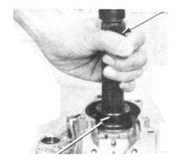
Install the crankshaft into the left crankcase.
