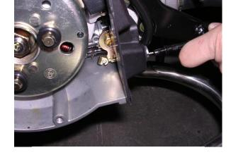
Check the O-ring, gear & seal for wear or any damage.
