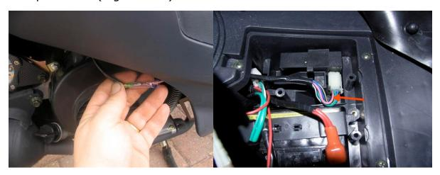
When you have disconnected this wire you will need to cover the ends with the electrical tape. **DO NOT DISCONNECT ANY OTHER WIRE.** The pink wire sends information about the speed of the back wheel to the CDI unit. If the CDI unit doesn't receive this info (because we disconnected it!) it thinks you are not moving and will allow the engine to go to full throttle.
