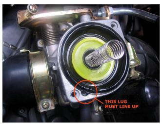
Now you need to put everything back together. Replace the black rubber seal and tube into the carb first. When you do you will need to ensure that the small lug is lined up with the recess in the carb top, and that the seal is seated correctly.(See Photo Below)
