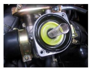
Now Carefully remove the rubber seal and the yellow disc will come with it. Inside this part there is a white plastic 'Plug' and a metal needle two small washers on it. One is loose and will fall off never to be seen again, if your not careful, and the other is fixed to the pin in a groove at the top. There should also be a small rubber
