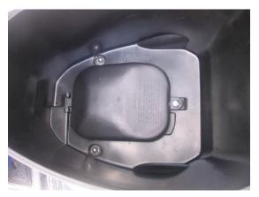
Opening this cover by removing the silver screw will give you access to the Carburettor.
