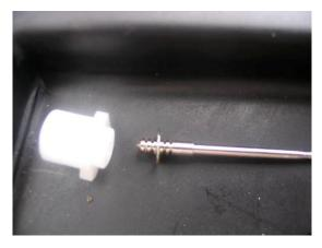
Now you need to remove the fixed washer. You can do this by using the pliers to pop the washer off. Be sure not to bend the needle, it is easy done and would make it unusable! The washer now needs replacing onto the needle, but now, place it onto the middle groove. See photo
