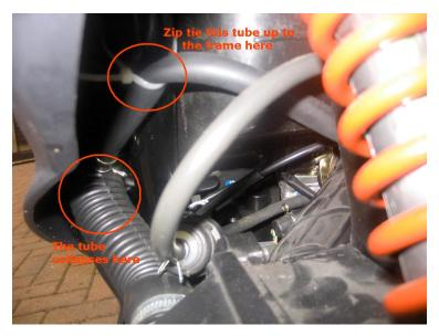
You can do this a couple of ways. You could place a plastic tube inside the hose to stop it collapsing or you could 'zip tie' the smaller tube to the frame, again stopping it from collapsing. I tied the small tube to the frame, see photo.
