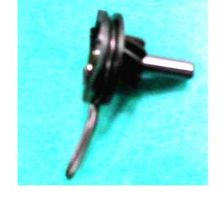
Check the wear & damage of starting shaft , bearing and driving gear.
