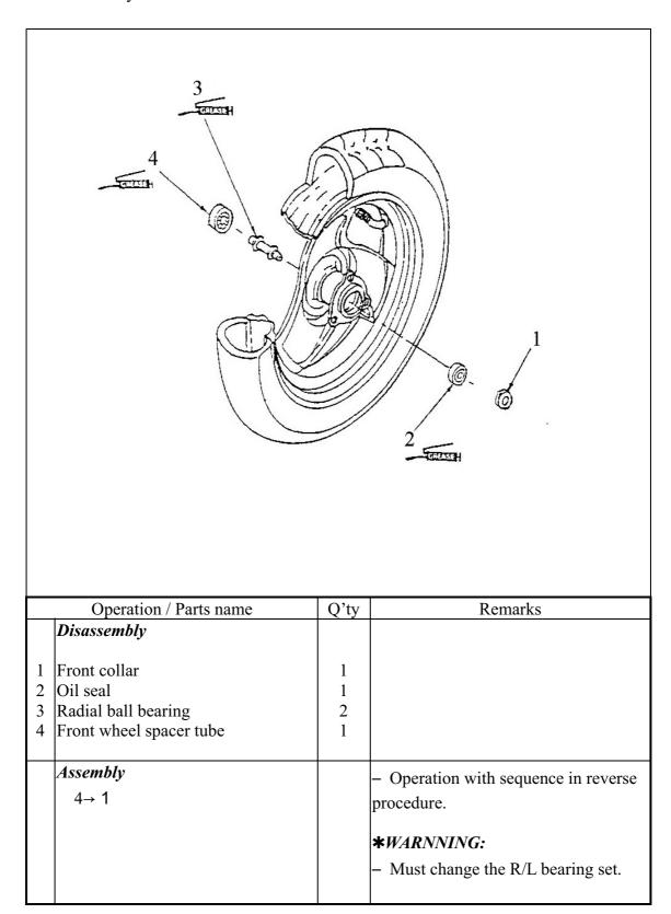
Assembly / Disassembly of Front Disk Assembly / Disassembly of Front Disk
